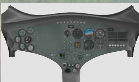
a panel for individual GPS installation,
