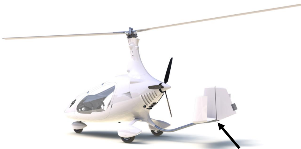
Fig. 2 – Installation point for Skid Plate rear
