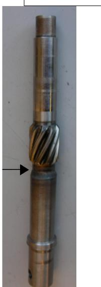
Action required. - Replace Bendix gear pinion.
