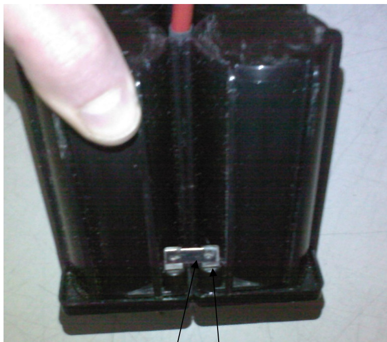
Link at the base of the battery
