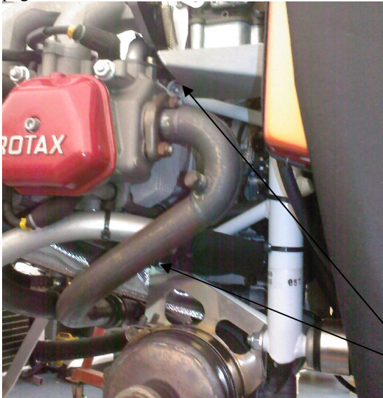
Engine bearer bolts (2). Same on engine right side.
