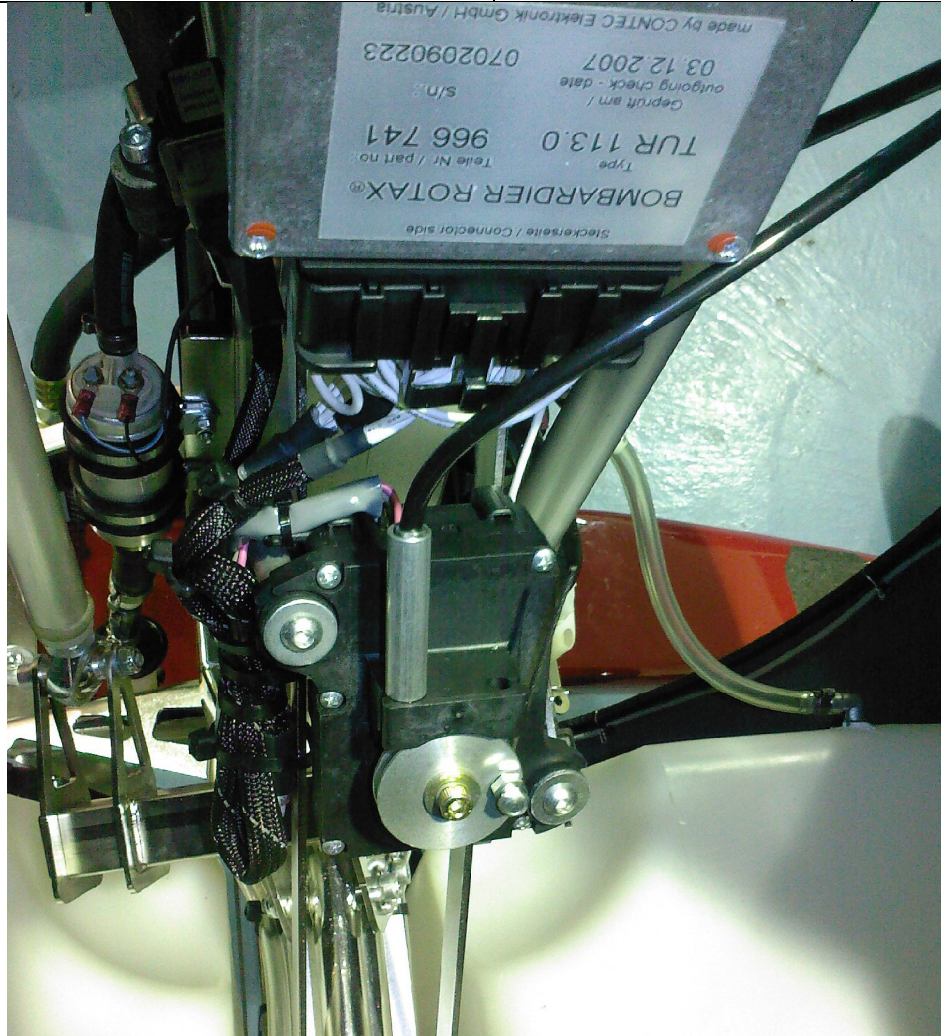
Waste gate control mounted on the straps, cables tied to right side as shown
