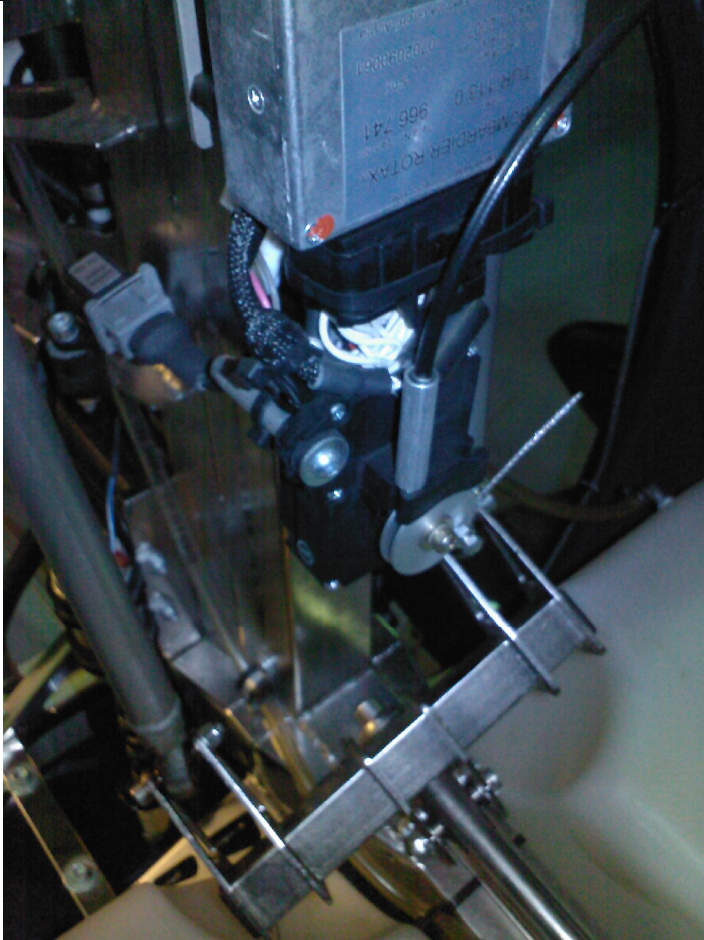
View of original turbo waste gate control unit attachment.
