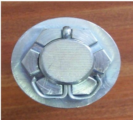
Top view of rotor bearing nut with split pin fitted.
