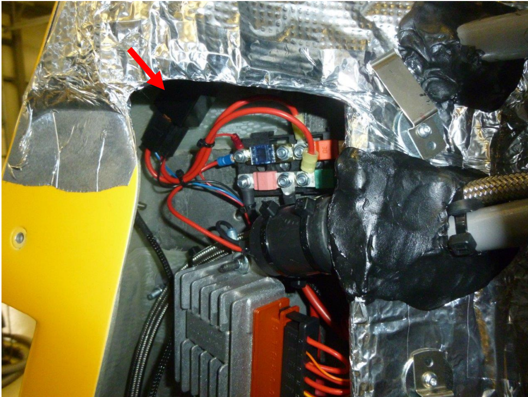
Fig. 3 – Position of the fuel pump relay (Cavalon)
