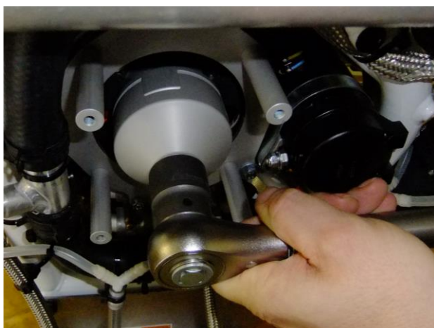
Fig. 5 – Torque dog gear with 140 Nm
