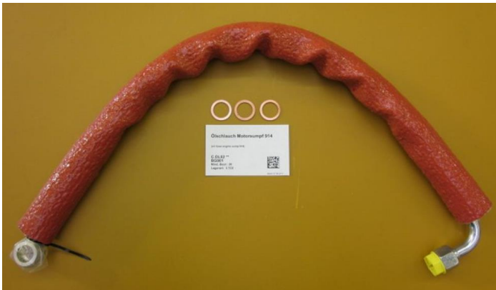
Fig. 2 – Rubber ,oil hose engine sump' (to be replaced/old)
