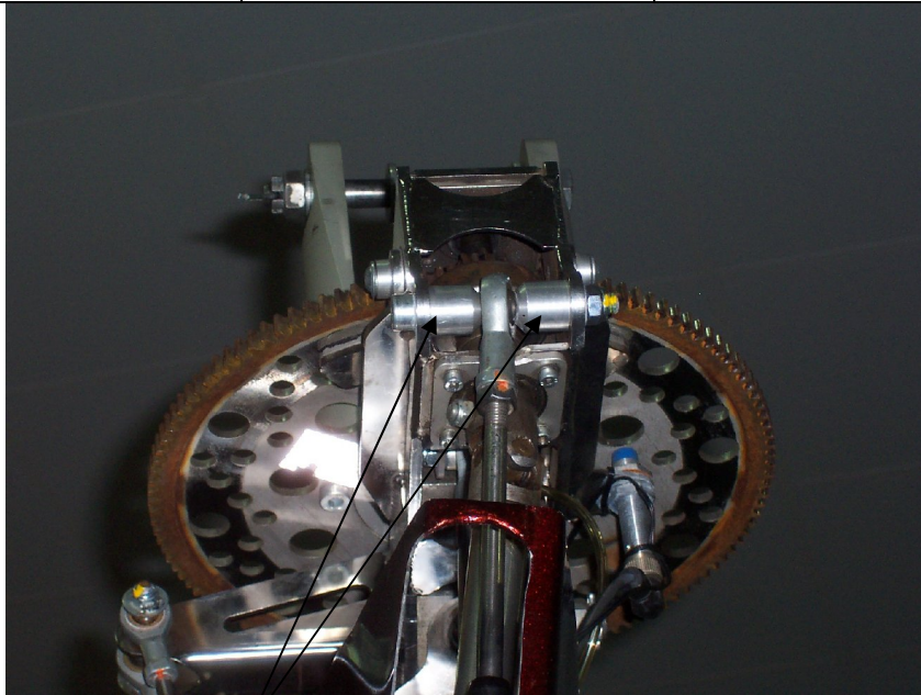
19mm conical spacers either side of pitch control cable
