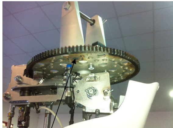
Welded plug at 11-o'clock position to rotor axis
