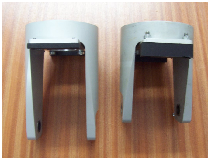
The different teeter-towers and teeter stops. Rotorsystem II (red end-caps) is used with the taller tower shown on the left An original rotor (orange end-caps) must NEVER be fitted to the taller tower
