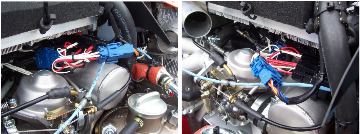
Relay module connected into wiring loom
