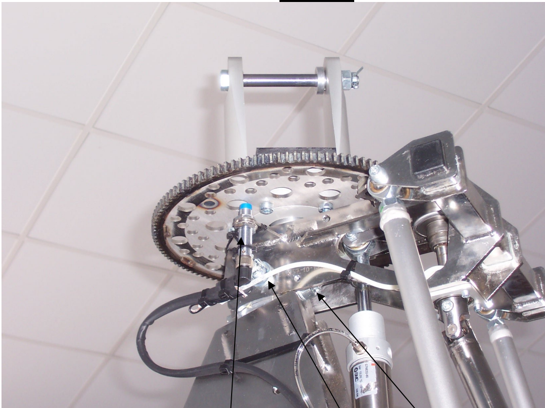
View of MT series rotor head. Speed sensor Pitch bolt Roll bolt
