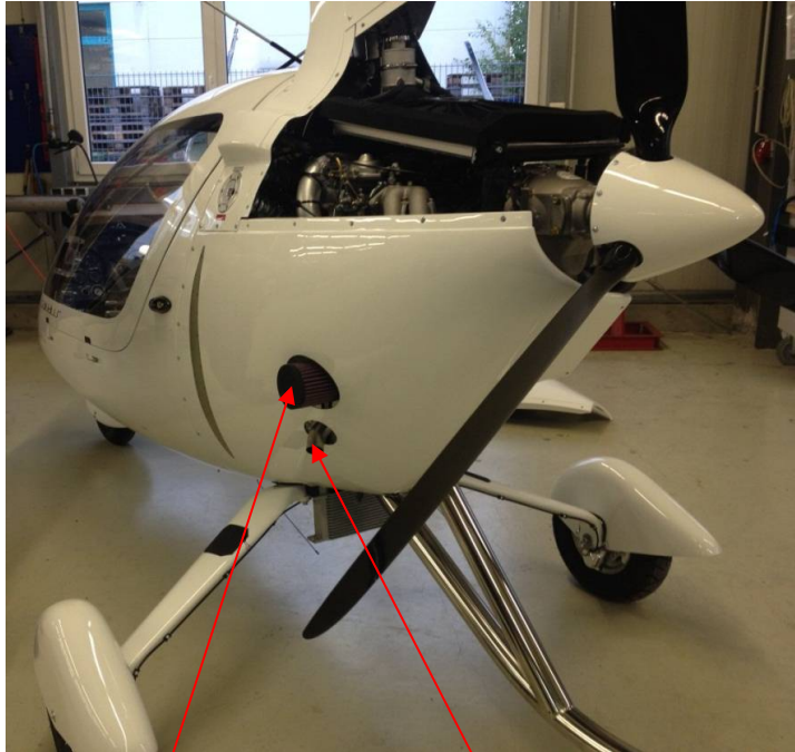
Intake after modification
