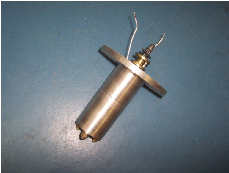
Motor/gearbox assembly removed
