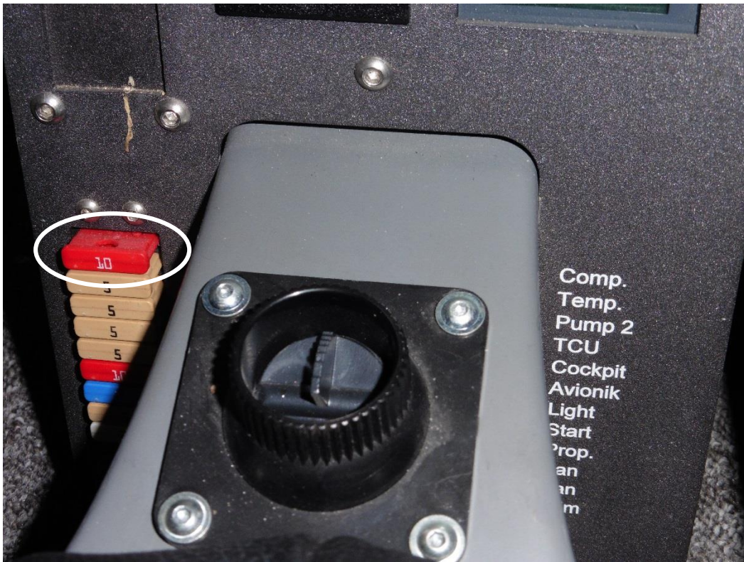
Fig. 1: 10A Fuse Compressor
