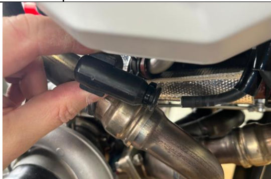
▲ Unscrewed spark plug cap
