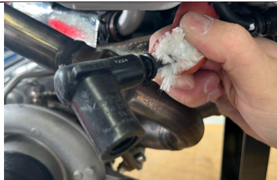
▲ Heat protection and spark plug cap
