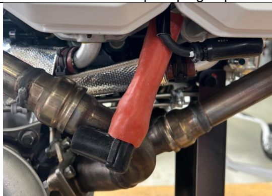
▲ Heat protection slid onto the spark plug cap
