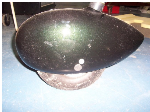
Blanking grommet in place
