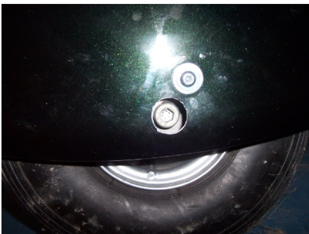
Hole cut into moulding
