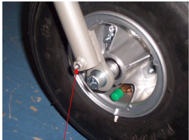
Attachment at fork fabrication
