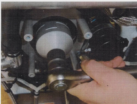
Fig. 5 - Torque dog gear with 140 Nm
