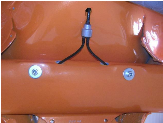
Front fasteners viewed from underside
