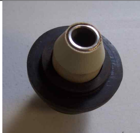
Sleeve fitted inside engine rubber with inner steel sleeve fitted
