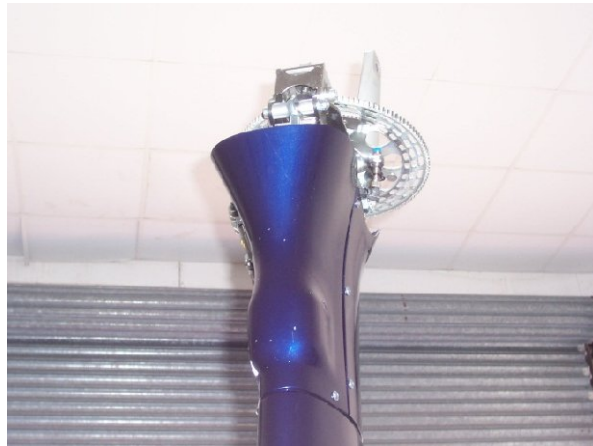
Two-piece mast cowling with vertical joint each side
