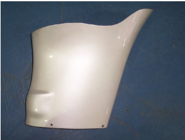
Single piece mast-cowling with split at rear
