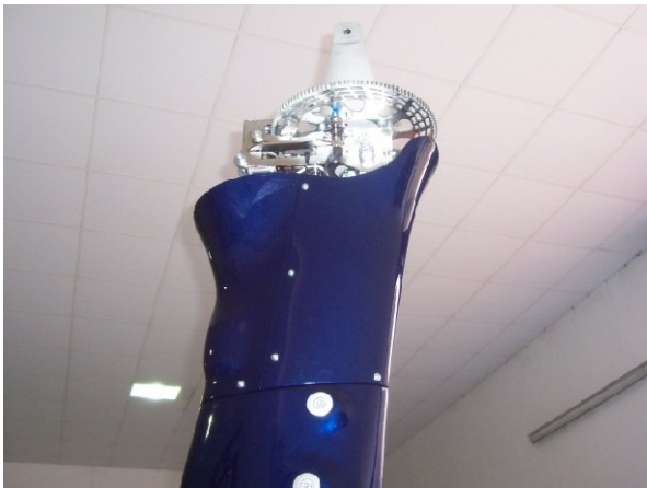
Two-piece mast cowling with vertical joint each side
