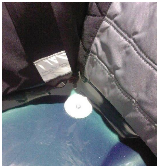
Large diameter washer fitted, rear front seat base bolt
