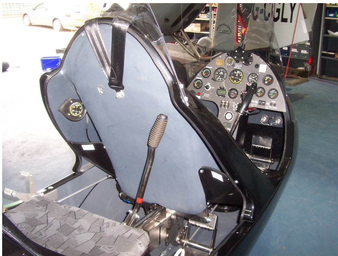
Pockets shown fitted to an instructional aircraft with longer control stick and additional ASI
