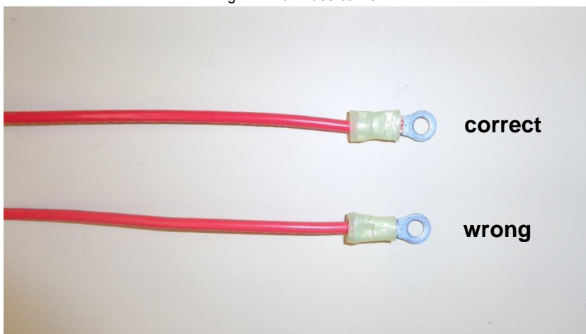
Fig. 2 – Crimp connection correct/wrong (outside)
