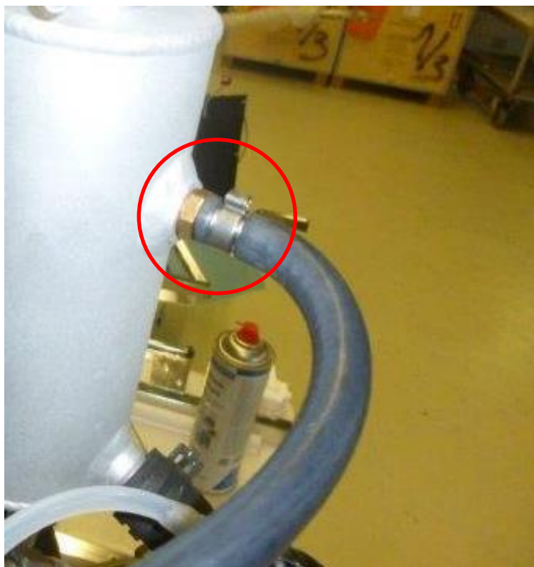
Fig.4: Nipple with copper washer and crimp
