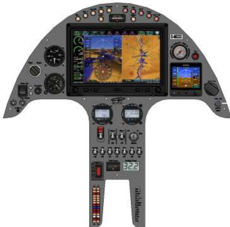
Example dual Garmin G3X/G5 installation
