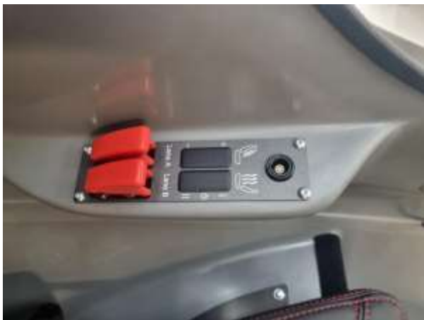
Rear seat headrest mounting and seat heating with instructor kill switch option fitted.
