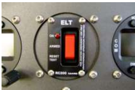
Remote cockpit switch
