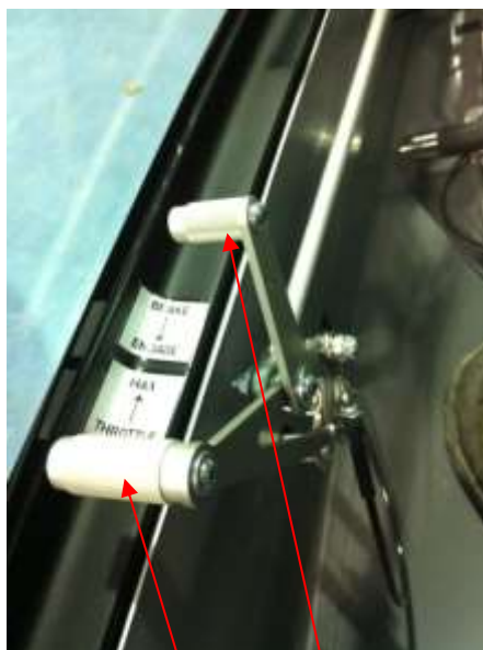
Throttle Brake Rear seat throttle and brake instructor pack
