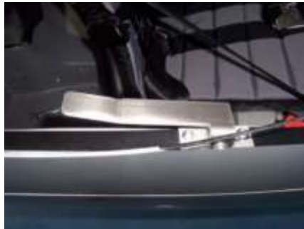
Inside-only lever for semi-open canopy
