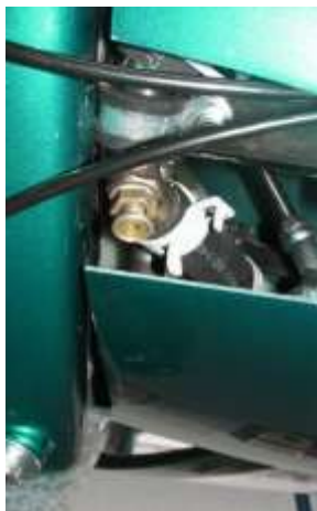
Photo showing water drain point, rear of the suspension bow
