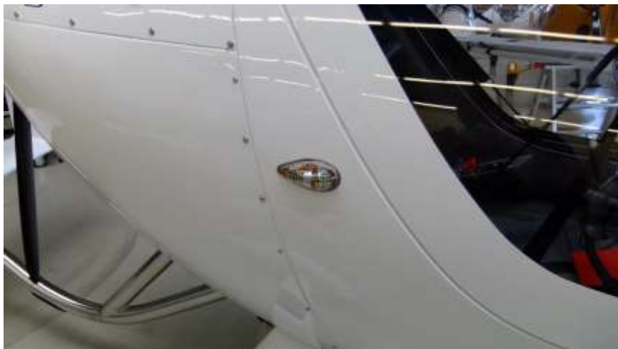
Certified nav and strobe unit, body mounted.
