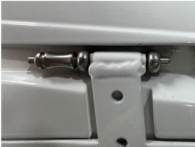
View of the door hinge pin. Note direction of pin fitment.
