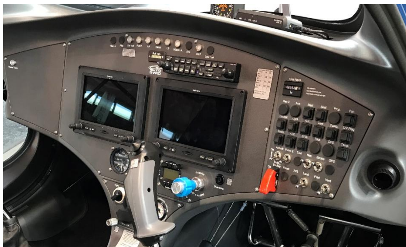
Example of panel from Cavalon 915iS/916iS with blue propeller control fitted (and dual panel Garmin G3x).
