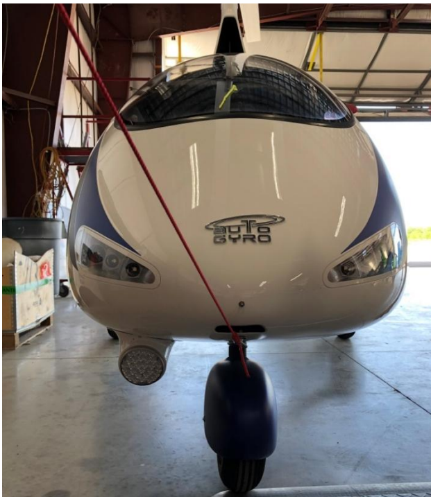
View of forward facing lamps with optional underbody landing light
