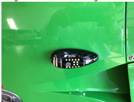
View of uncertified AutoGyro navigation and strobe lamp, for day conspicuity only.
