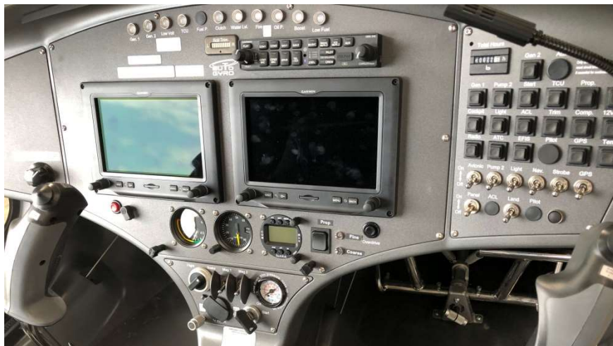
Example dual G3X installation
