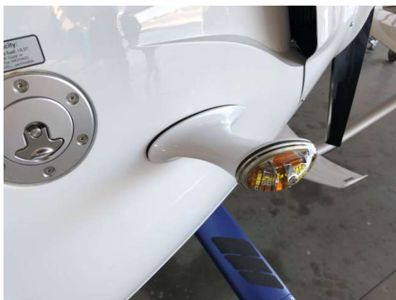
View showing stalk-mounted certified navigation and strobe lamp
