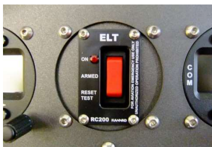
Remote cockpit switch
