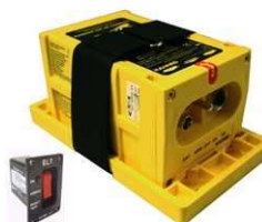
ELT transmitter and cockpit switch
