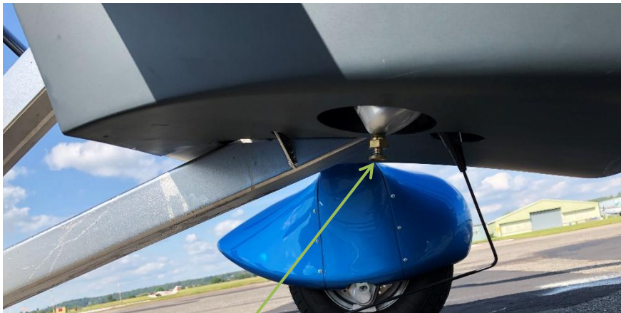
Location of gascolator drain point
