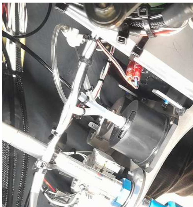
Figure 2 – Example for static lines, disconnect clear hose from instruments and use compressed air
