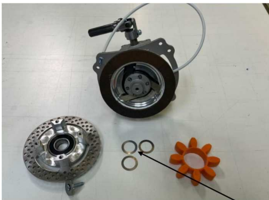
Figure 2 – Central screw and friction plate removed with previous installed shim washers
