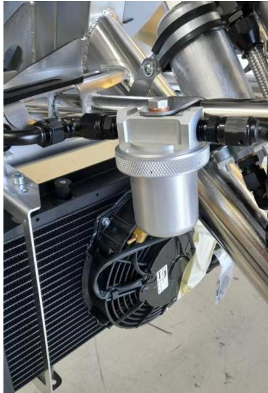
Figure 1 – Location of gascolator drain point.
