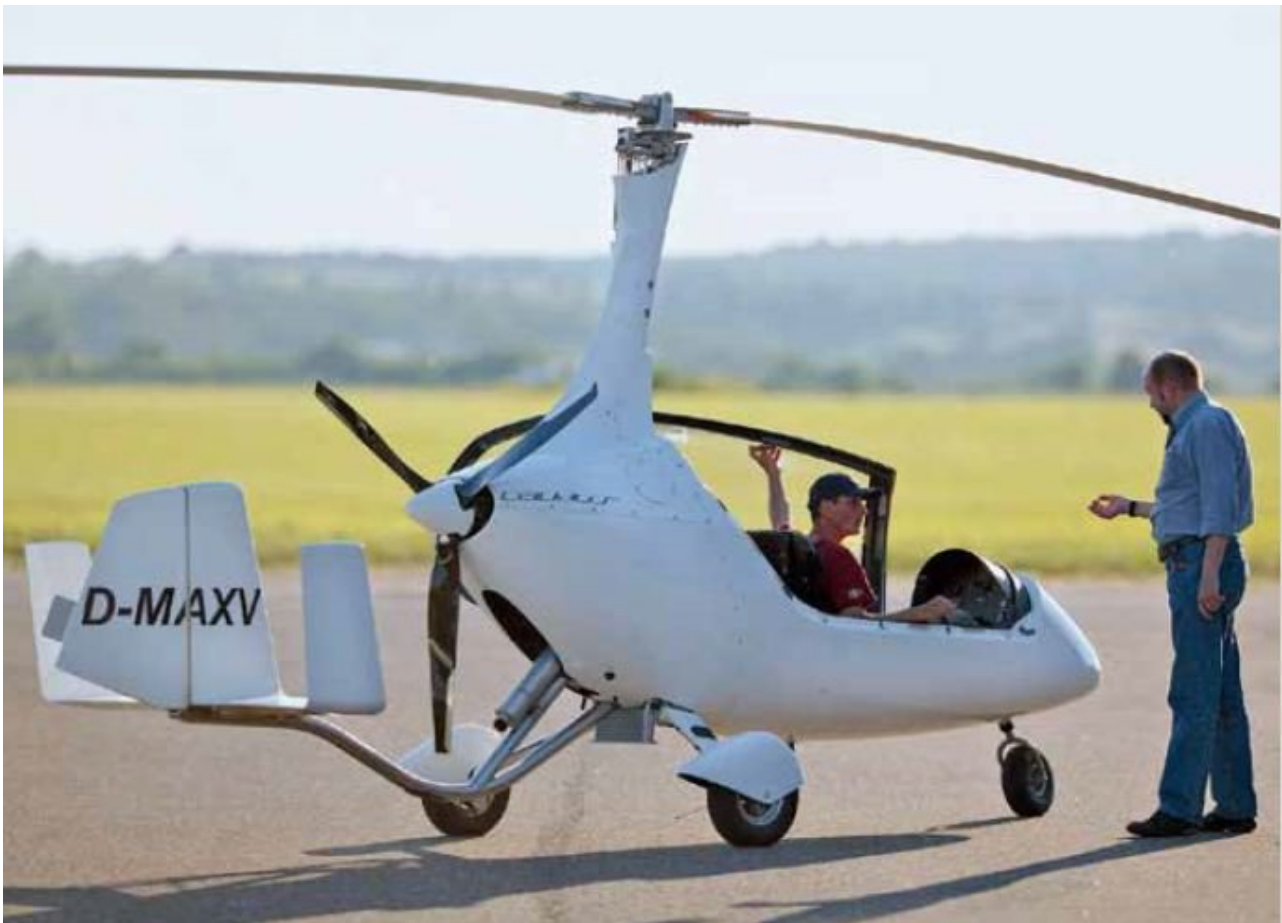
Calidus fitted with IVO-prop variable pitch propeller
