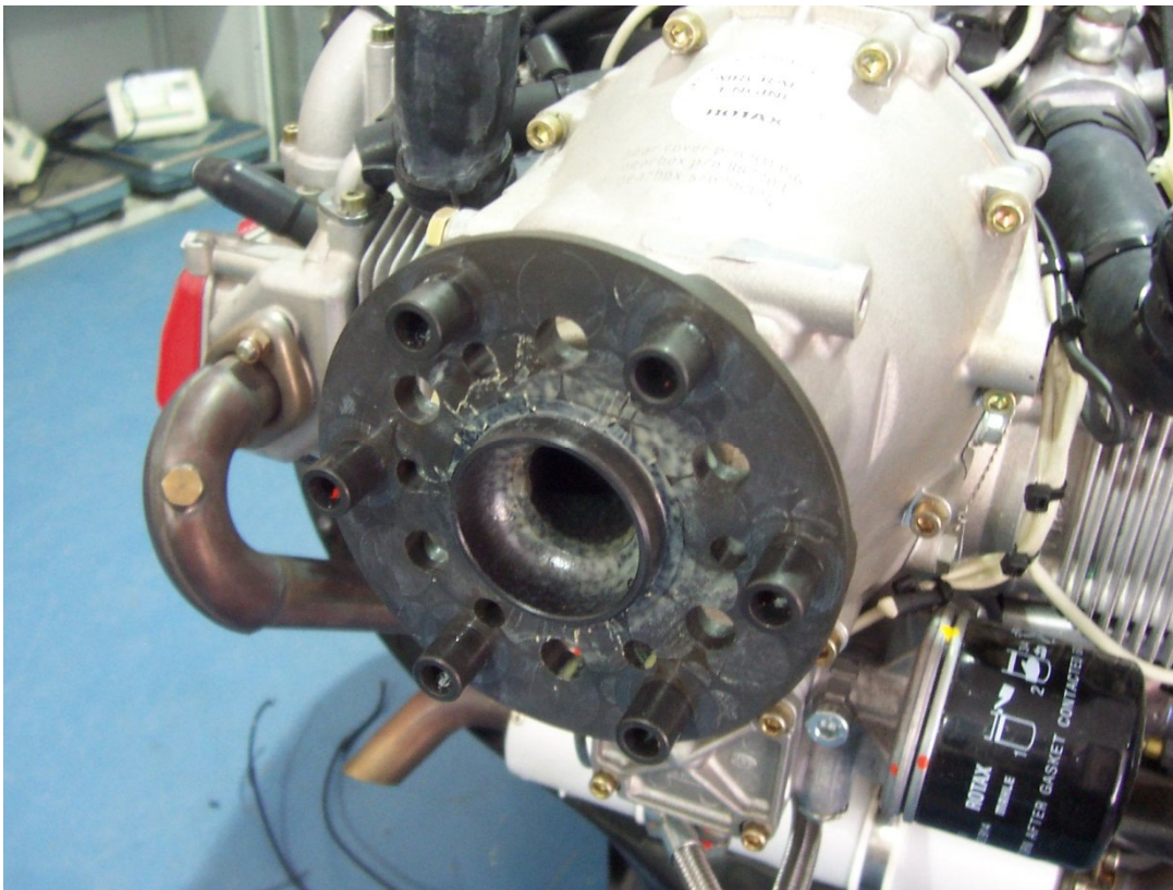
Engine gearbox flange with Rotax flange nuts fitted
