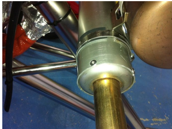
Silicone strip fitted under band-clamps (MC-193 / SB043)
