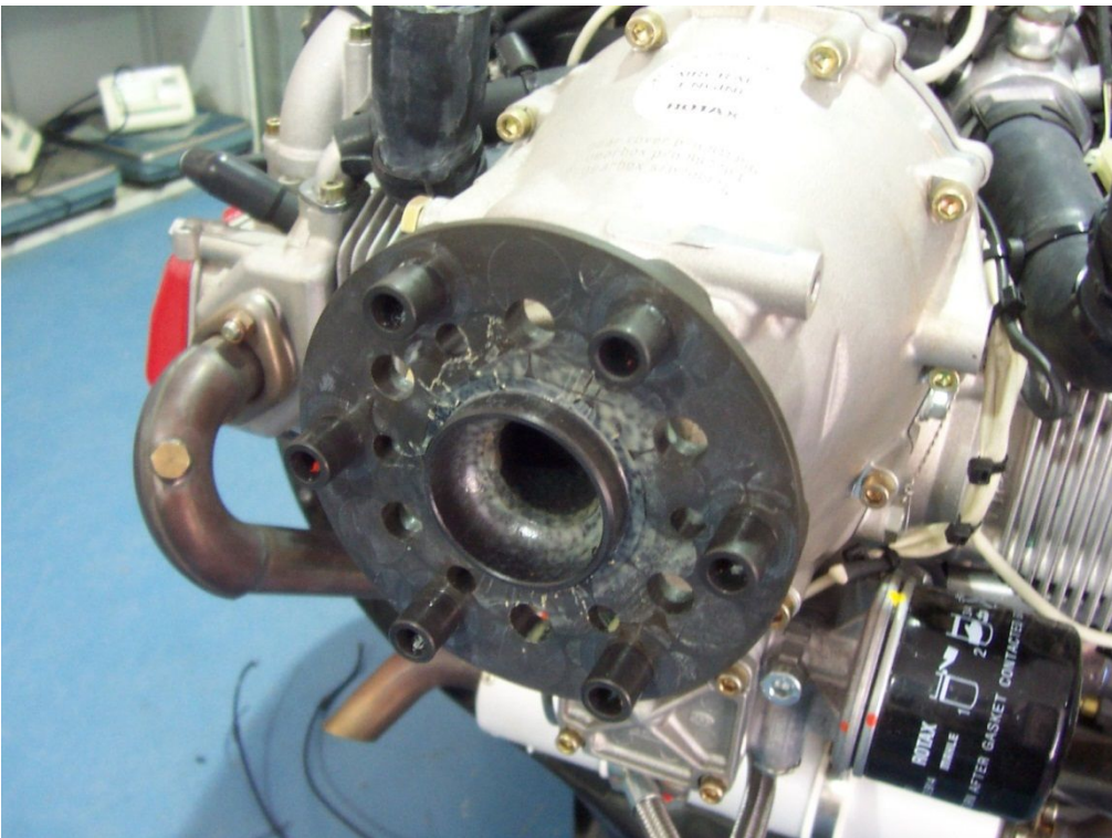
Propeller mounting flange with "torque-bushes"
