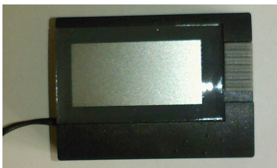
View of front, prior to panel fitment. Unit is bonded to panel. Switch should be down – this changes the unit between deg C and deg F
