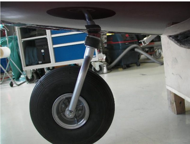
Nosewheel in place. Lubricate fork axis with W2000 grease or equiv during assy.
