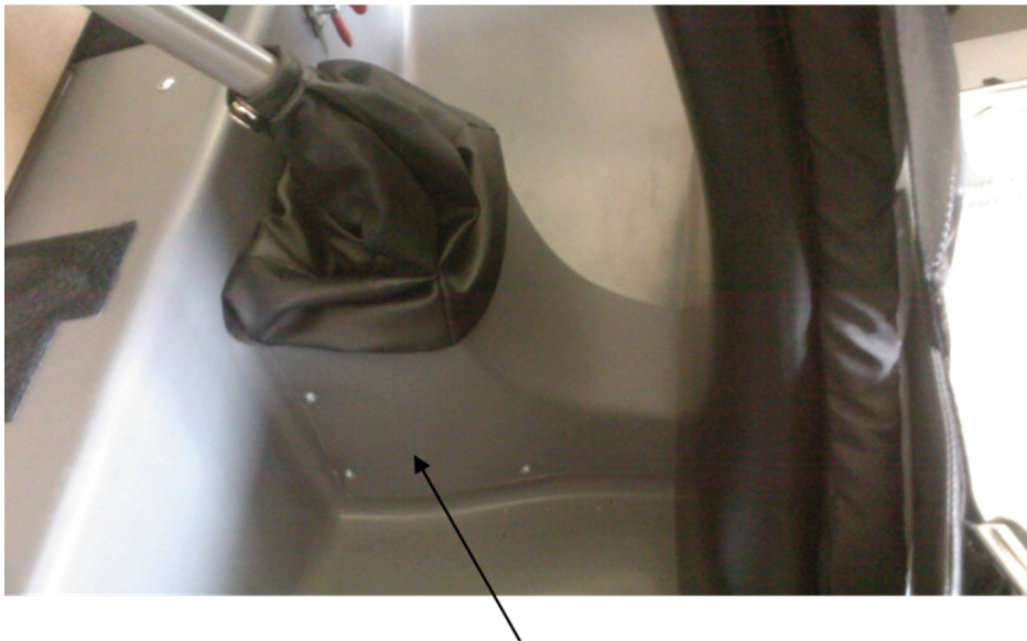
Cover, held in place with M4 screws
