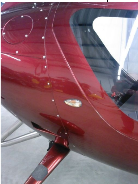
Aveoflash side strobe location (same for Skyflash)
