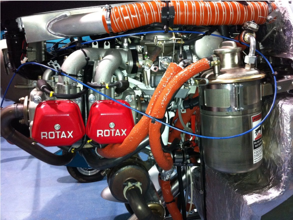
914UL engine right side installation
