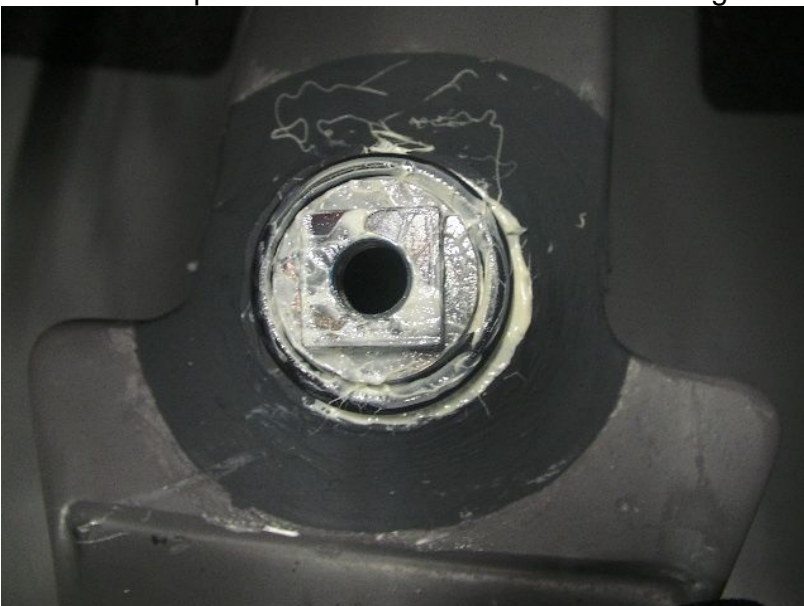
Top of fork tube has a square drive welded in which locates into the connecting plate. Note O ring fitted around shaft.
