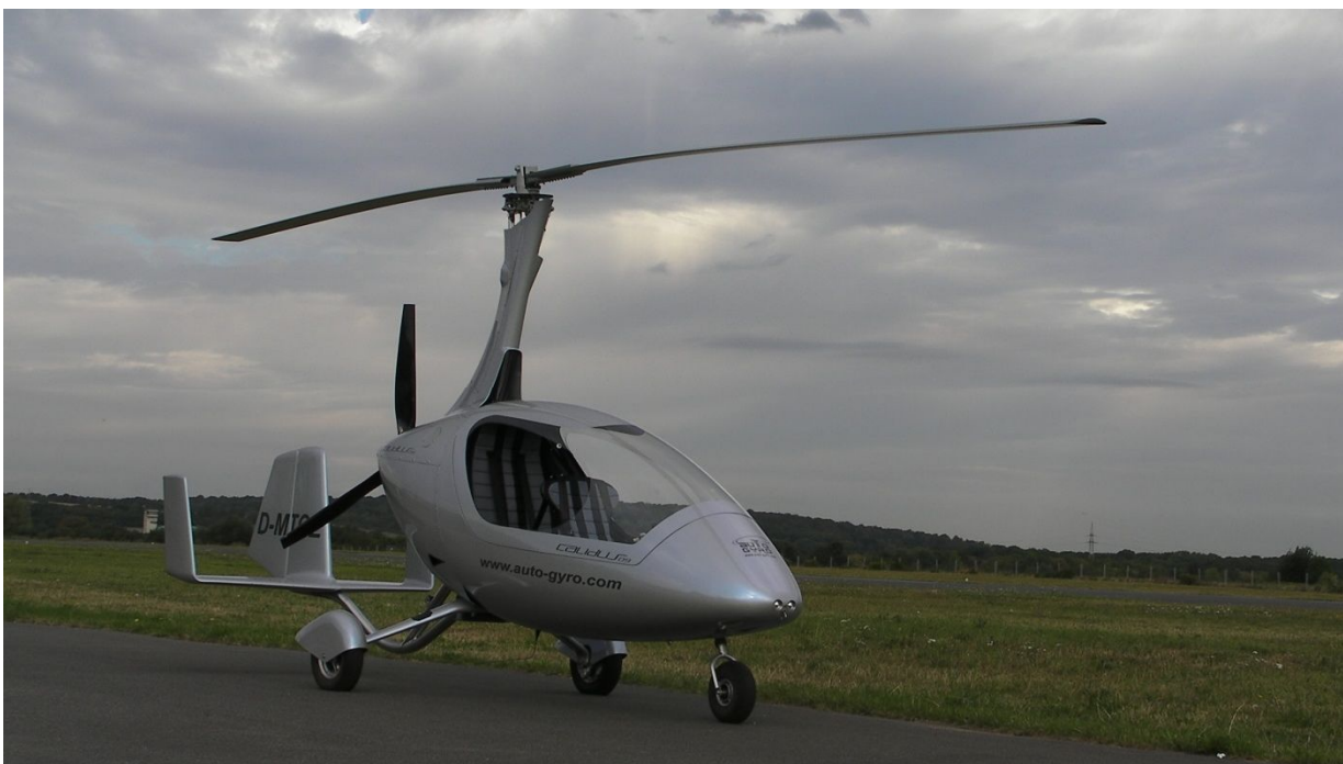
Calidus gyroplane, fitted with semi enclosed canopy
