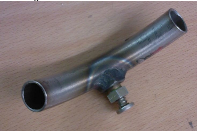
Fuel tank crossover tube with drain fitted.
