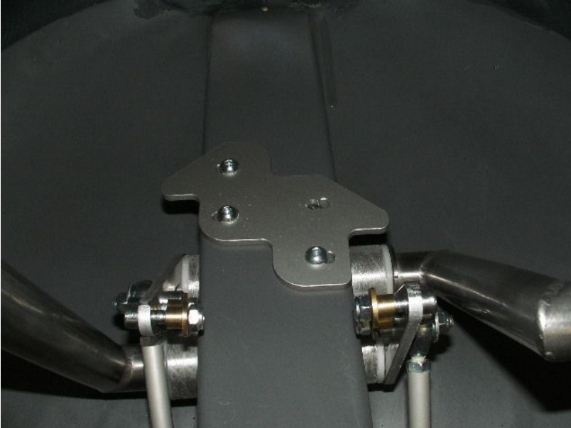
Pedal limit stop plate. Screws retained by loctite 243.
