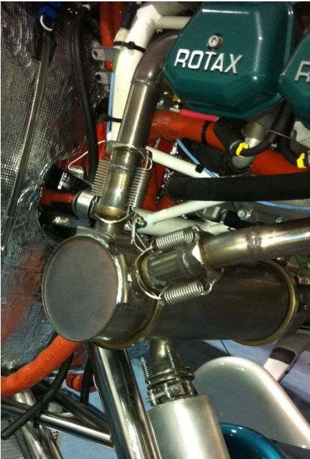
912ULS silencer & axial after muffler assy Springs are secured by cables for safety.
