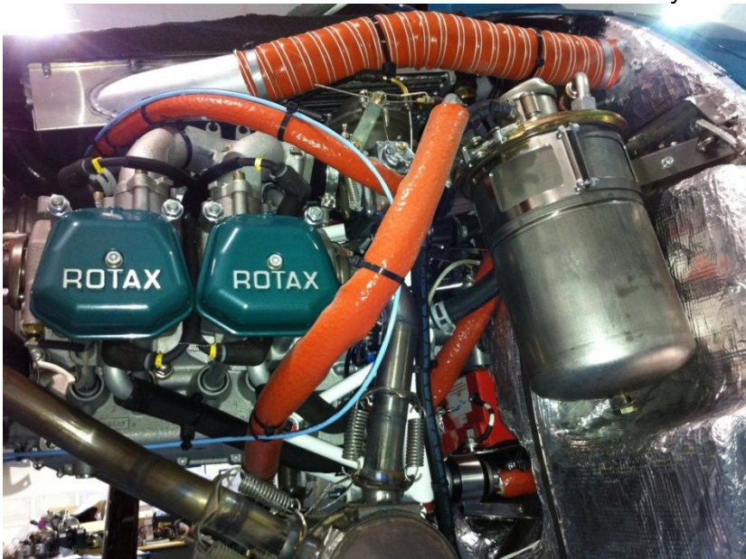
Left side, 912ULS engine. Take care that hoses are tied from the exhaust.
