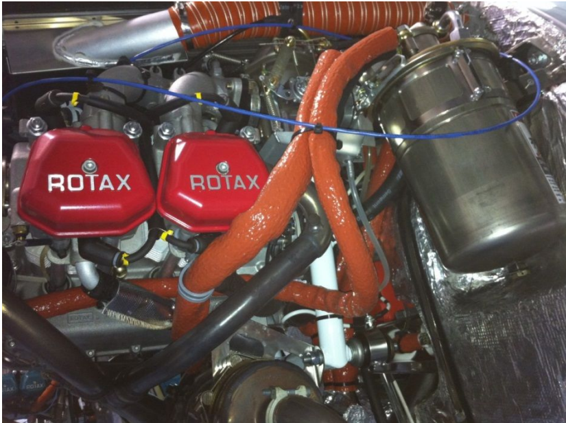
914UL left side hoses. Note that hose must be securely fixed to the engine.
