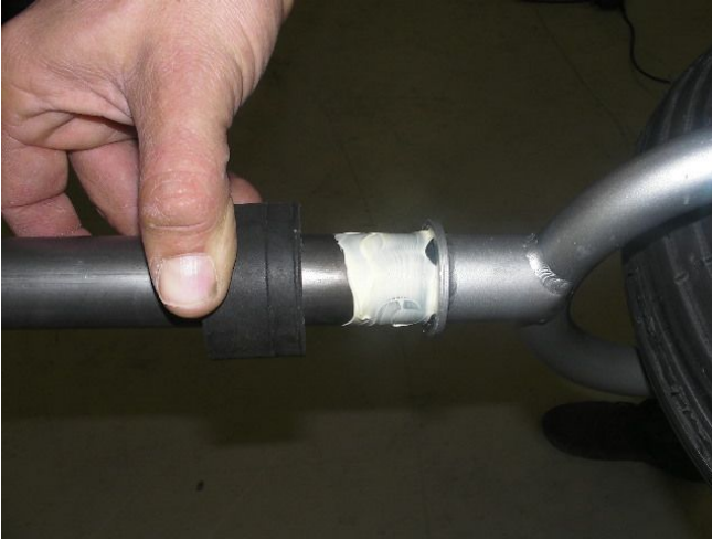
Suspension rubber for nosefork. Note grease under (W2000 or equiv axle grease)
