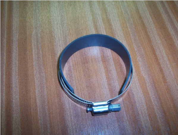
Silicone strip fitted under band-clamps (MC-193 / SB043)
