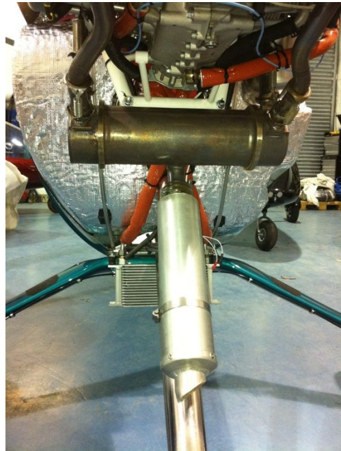
912ULS exhaust system with axial after-muffler
