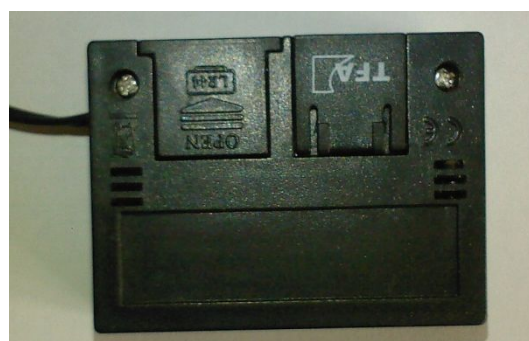
View of rear, showing battery slot for LR 44 (SR44 battery recommended for longer life)
