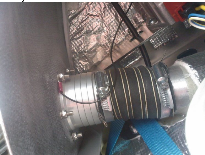
View of connection between tank and filler neck from under the cowl. Note the earth lead to the filler neck (hose is shown not covered in the fireproof sleeving)
