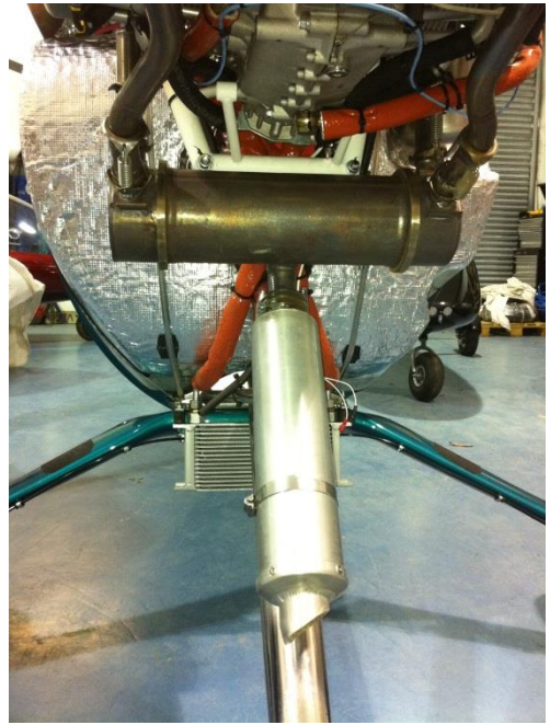
912ULS exhaust system with axial after-muffler
