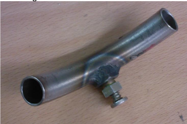
Fuel tank crossover tube with drain fitted.
