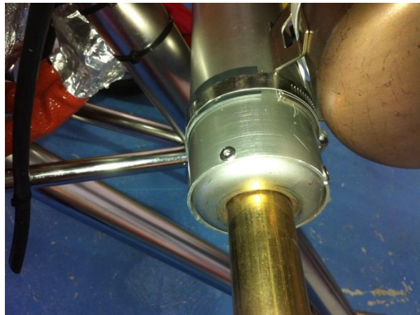
Silicone strip fitted under band-clamps (MC-193 / SB043)
