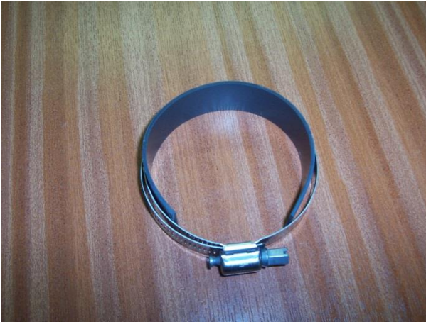
Silicone strip fitted under band-clamps (MC-193 / SB043)
