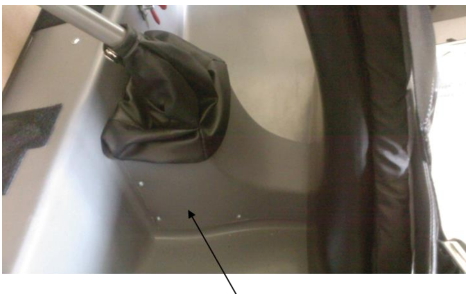
Cover, held in place with M4 screws
