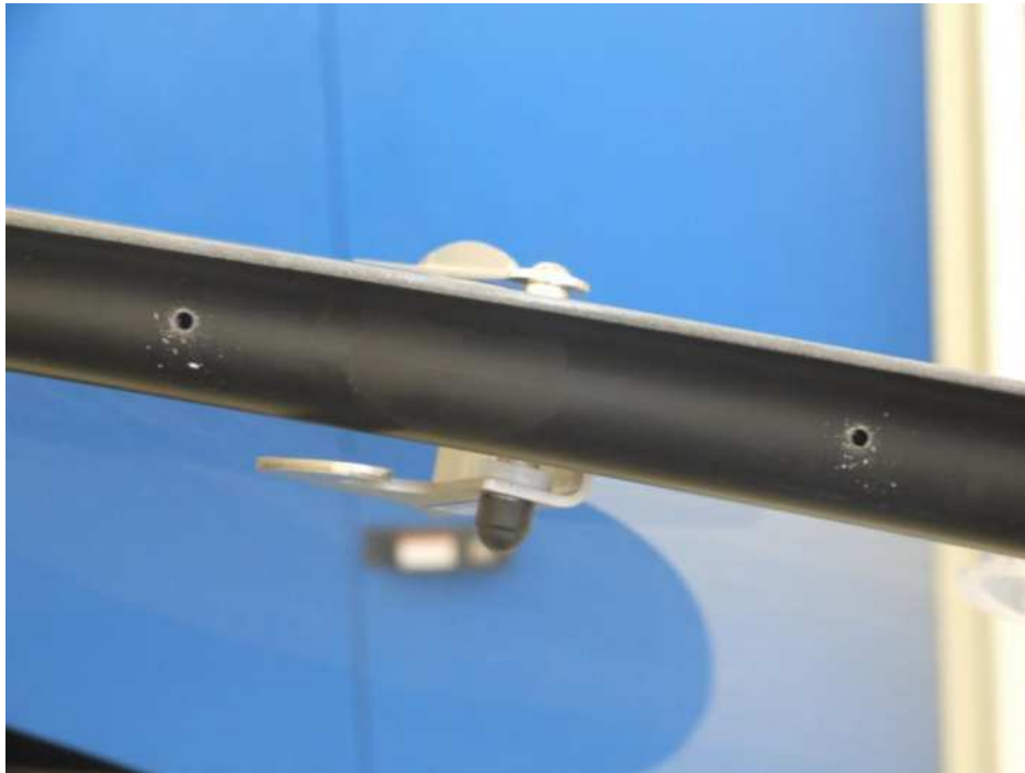
Figure 3 – Attachment bores drilled
