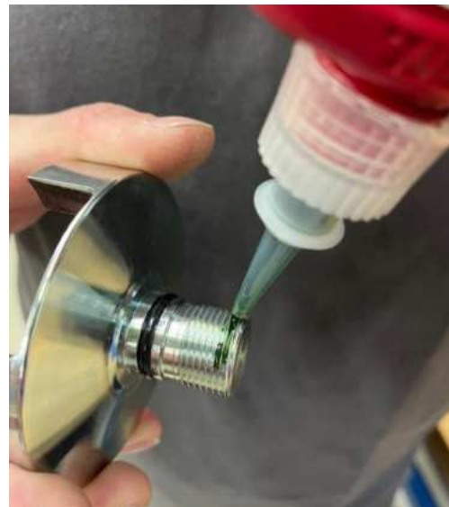
Figure 5 – Loctite onto thread
