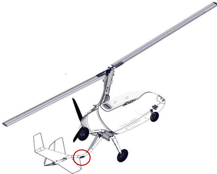
Figure 1 – Installation position of keel tube protection pad
