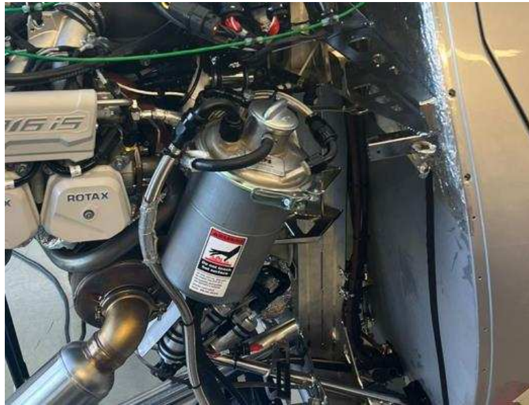
Figure 1 – Oil tank bracket removed
