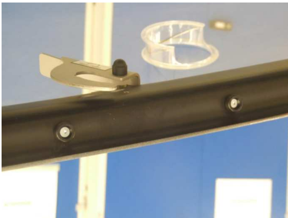
Figure 4 – Canopy spacers installed
