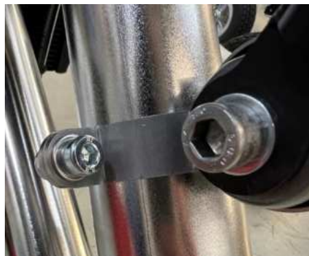
Figure 5 – Screws on the clamp on the keel tube
