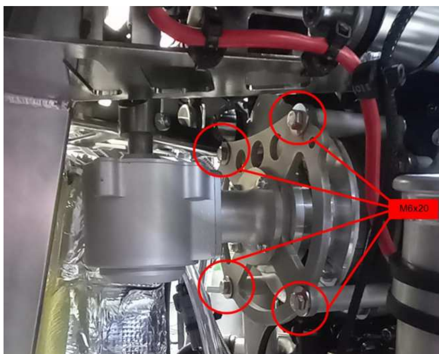
Figure 3 – Location of M6x20 screws (PN 45753)
