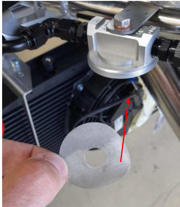
Figure 3 – Filter removed from Gascolator cap for inspection and cleaning
