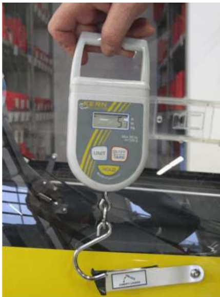
Figure 1 – Measurement on canopy lever breakout
