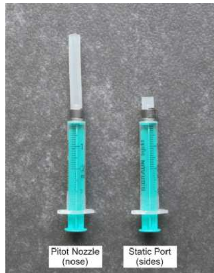
Figure 1 – Pitot static integrity test equipment
