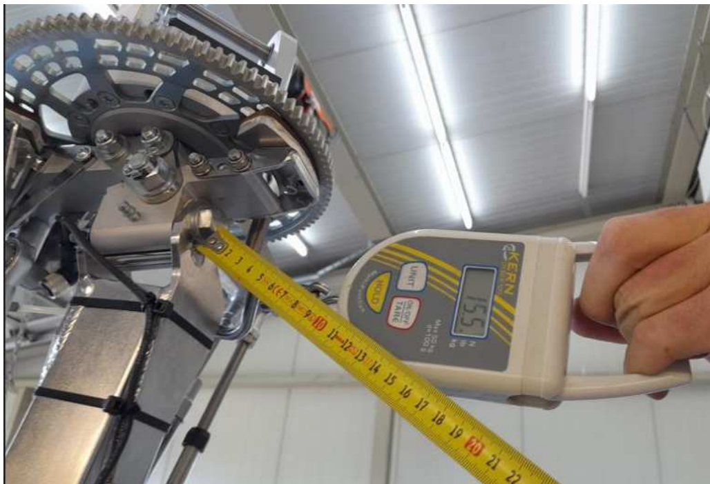
Figure 3 – Force applied in flight direction
