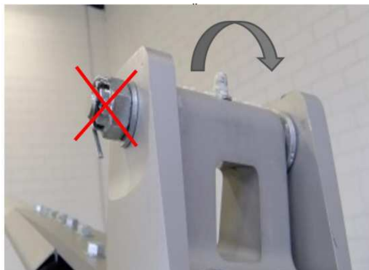
Figure 4 – bolt is not allowed to turn if rotor system teeters
