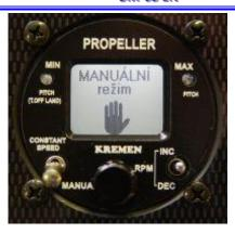
When switch (8) is in Constant speed position, turning knob (9) allows setting of TAKE-OFF speed.
