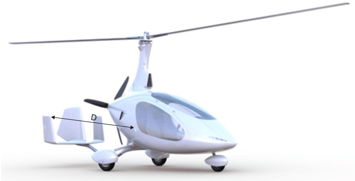
Fig. 1 - Measurement of Stabilizer Alignment (RH side shown)
