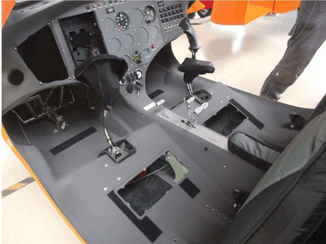
Fig. 1 - Service covers below seats ('Equipment Cover')
