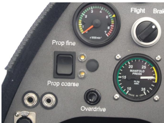
Fig. 5 - Rocker Switch and LED mounting position
