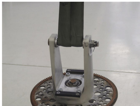
Lifting belt looped around teeter bolt
