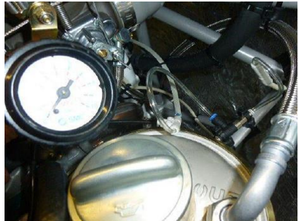
Fig. 4 - Connection between clutch and pressure reducer
