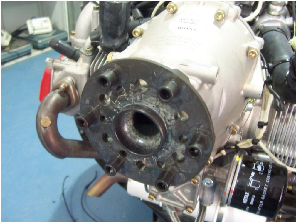
Propeller mounting flange with "torque-bushes"
