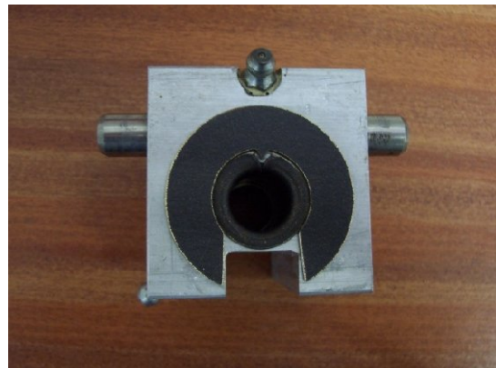
Slotted washer in place
