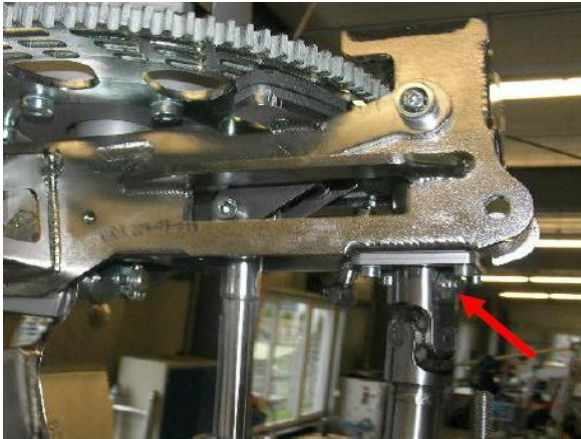
Fig. 1 - Upper pre-rotator drive connected to Bendix shaft
