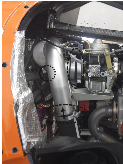
Fig. 1 - Clearance airbox to engine mounting frame (R914)
