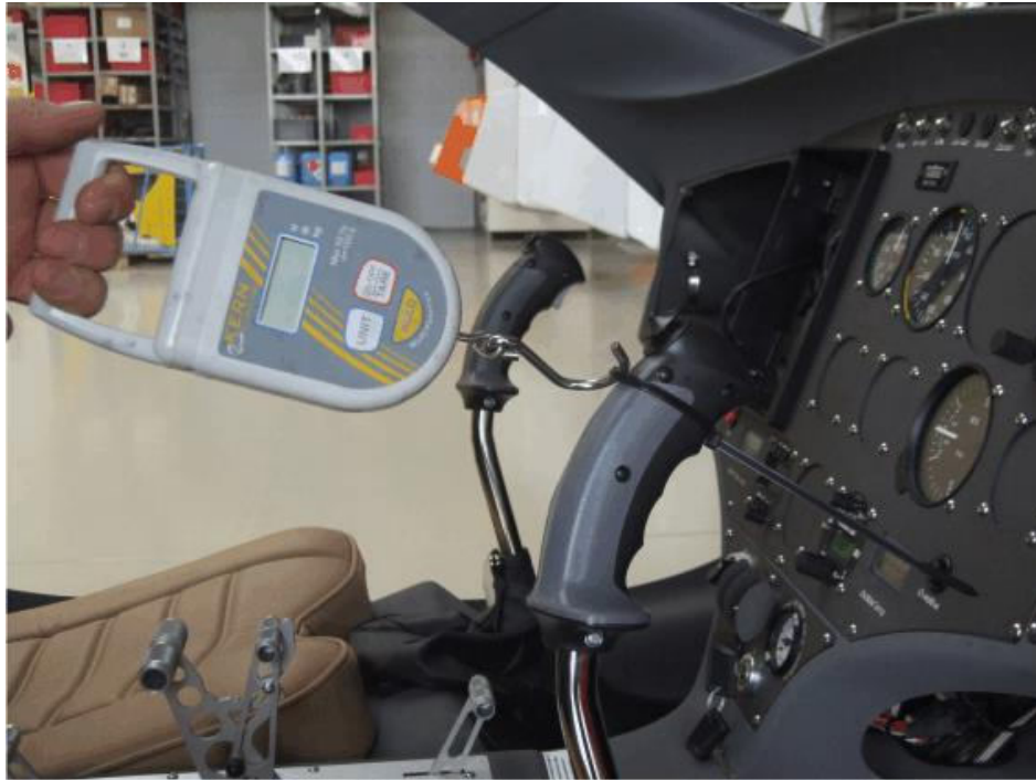
Fig. 1 - Measurement of rotor control friction
