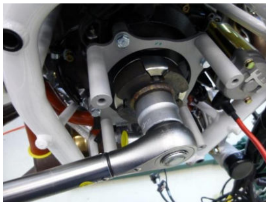
Fig. 5 - Torque dog gear with 150 Nm
