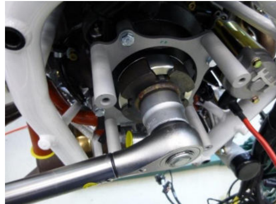
Fig. 4 - Tighten dog gear to 150Nm
