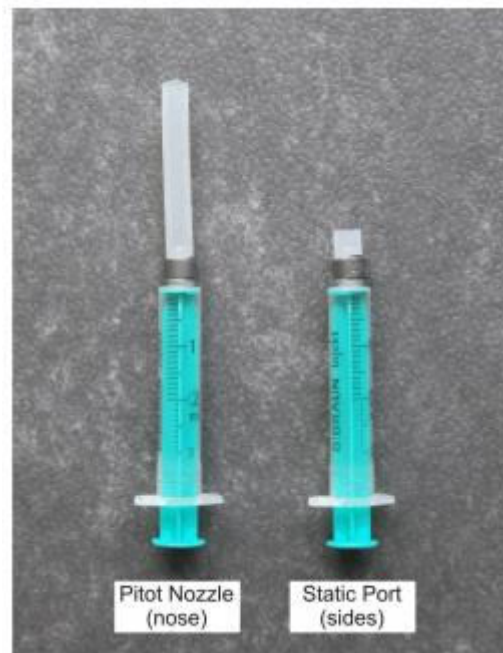
Fig. 1 - Pitot Static Integrity Test Equipment
