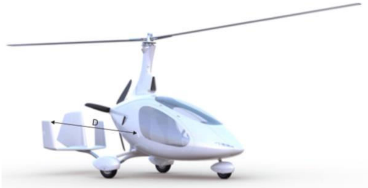
Fig. 1 - Measurement of Stabilizer Alignment (RH side shown)
