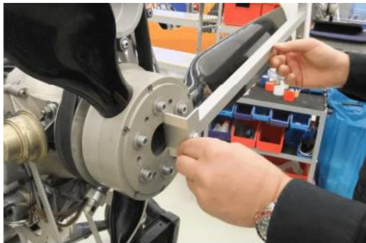
Fig. 2 - Propeller pitch adjustment and tool
