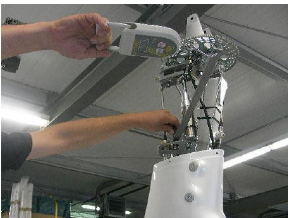
Fig. 5 - Measurement of breakout torque
