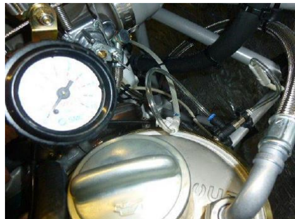
Fig. 4 - Connection between clutch and pressure reducer
