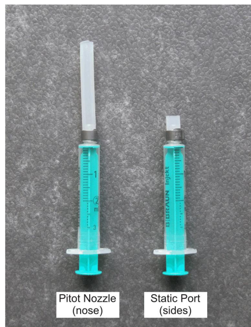
Fig. 1 - Pitot Static Integrity Test Equipment
