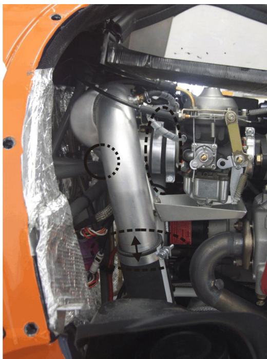
Fig. 1 - Clearance airbox to engine mounting frame (R914)
