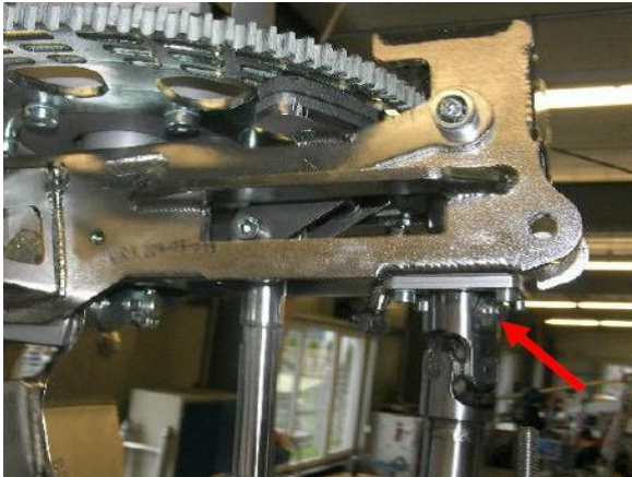
Fig. 1 - Upper pre-rotator drive connected to Bendix shaft
