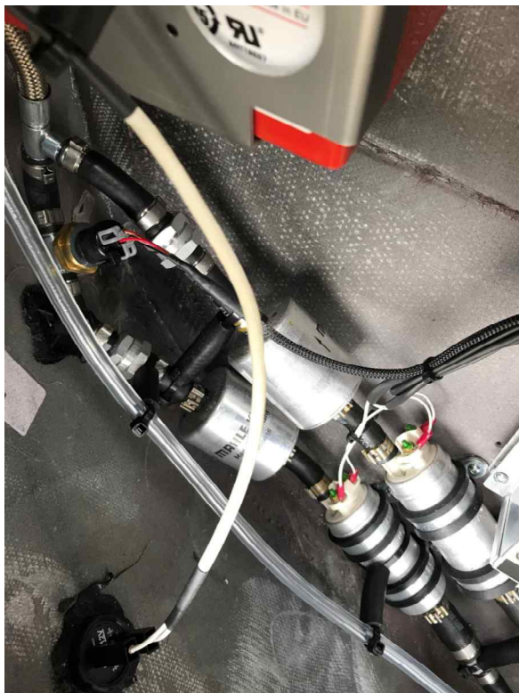
Fuel pressure sender integrated into fuel-pipes
