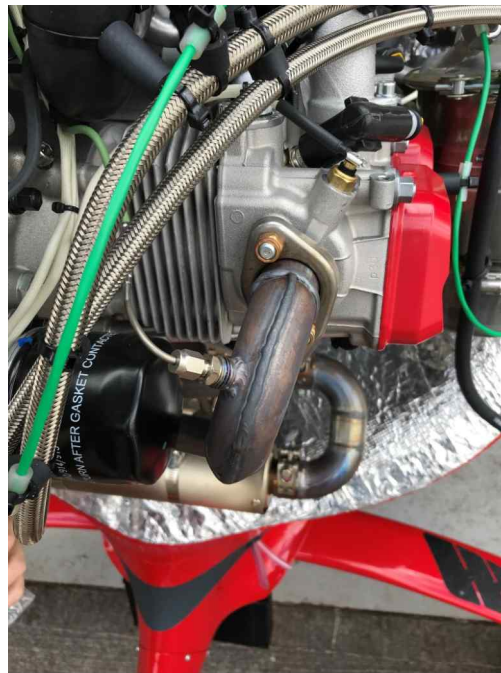
EGT sensors mounted into the standard Rotax sensor receptacles
