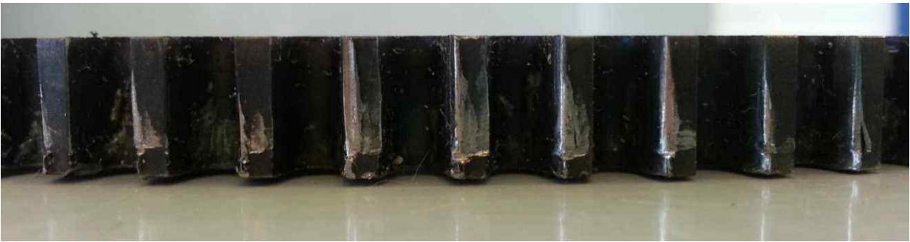
Wear Pattern (uneven)
