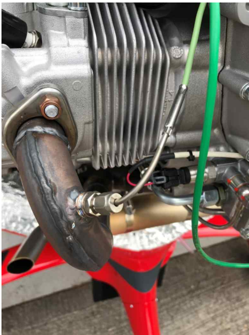
EGT sensors mounted into the standard Rotax sensor receptacles
