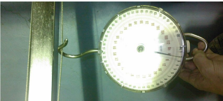
Apply a tensile load of 2Kg, and re measure gap. Cable should move between 8 and 24mm. Adjust turnbuckles as required.
