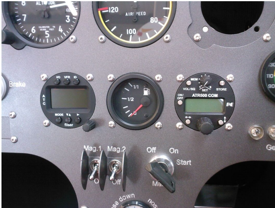
Float-driven (electrical) fuel gauge
