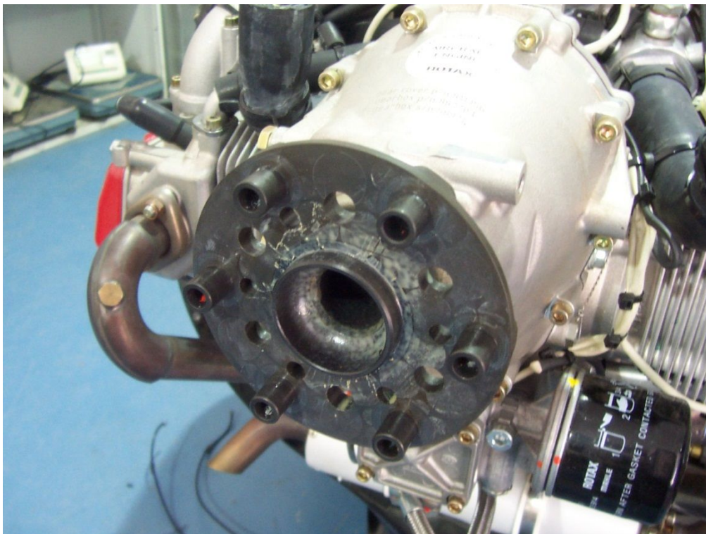
Propeller mounting flange with Rotax captive nuts fitted
