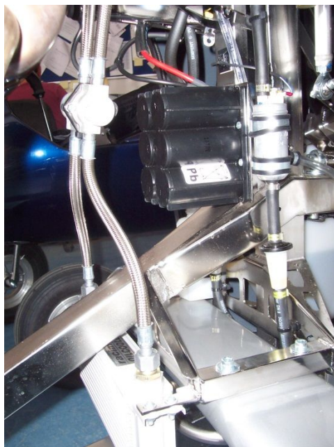
Braided hose construction and new oil thermostat
