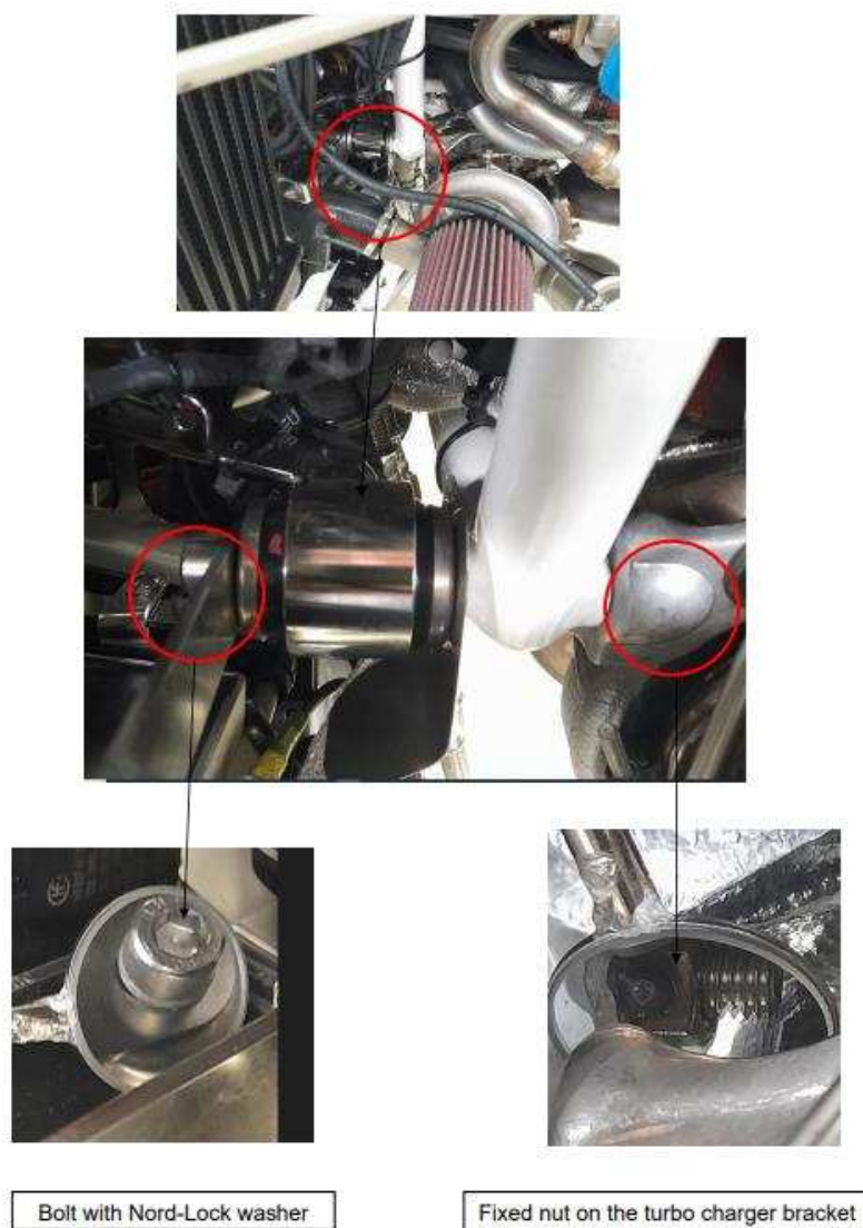
Figure 3 – 915 / 916 version with fixed nut
