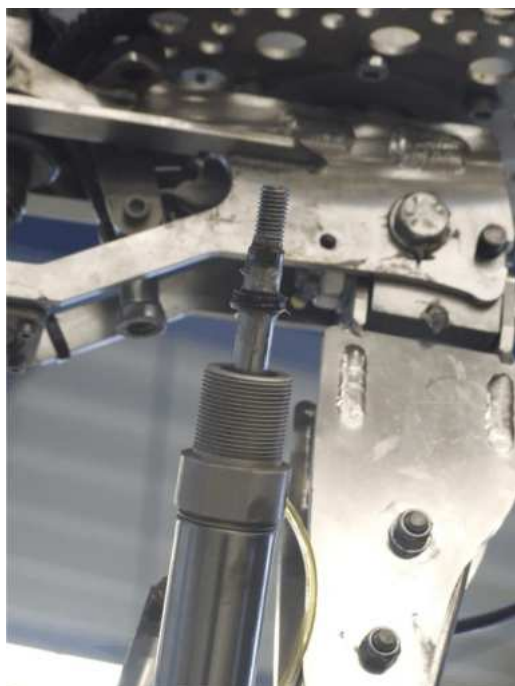
Figure 3 - New seal ring installed with special grease
