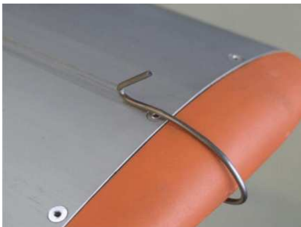
Figure 2 - Positioning of measuring cord
