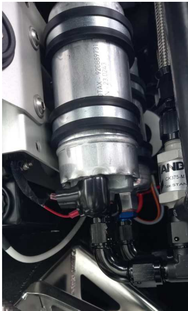
Figure 2 – Electrical fuel pump (916 engine)
