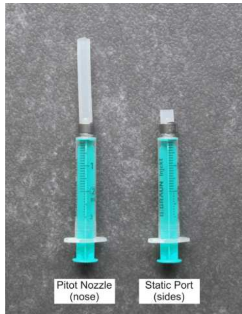
Figure 1 – Pitot Static Integrity Test Equipment Pitot Nozzle
