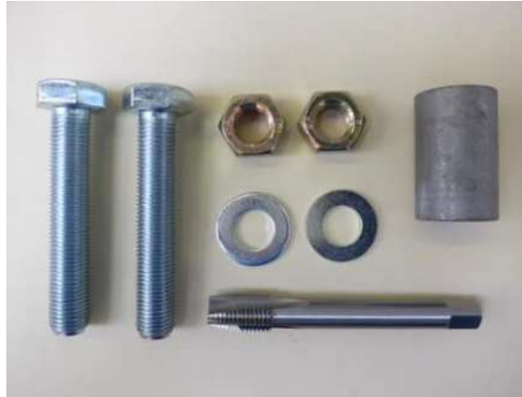
Figure 4: Bushing removal tool Teeter Block
