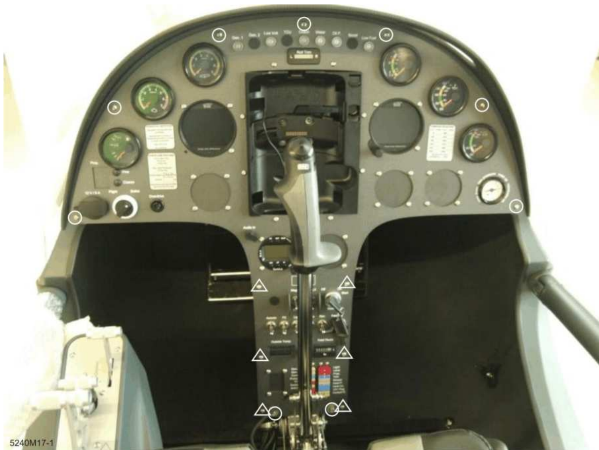
Figure 1 - Instrument Panel with attachment bolts
