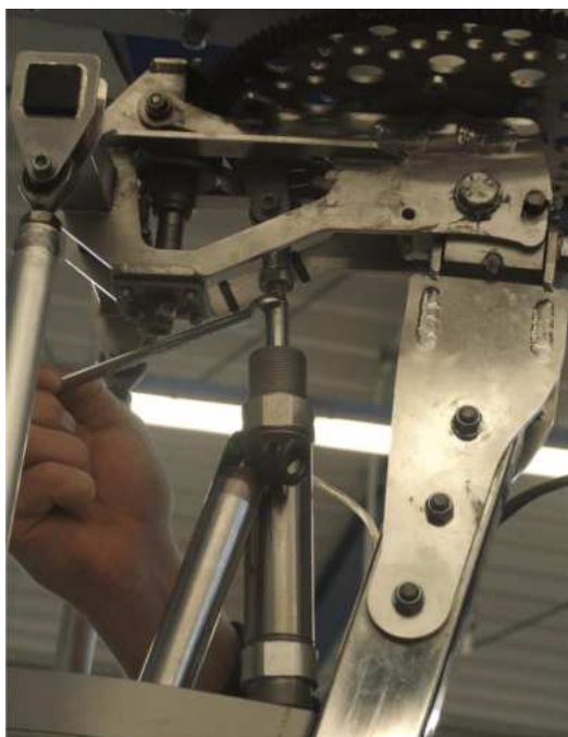
Figure 1 - Disconnect rod end from ball joint
