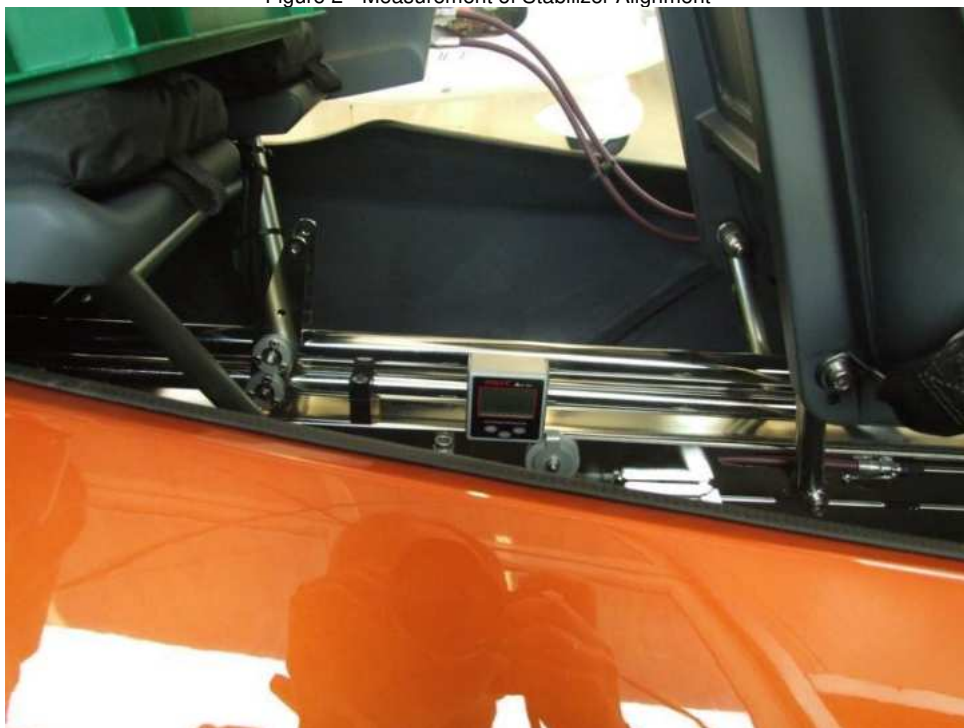
Figure 3 - Measurement of reference zero
