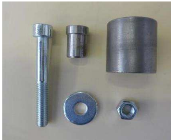
Figure 5: Bushing removal tool for Teeter Tower
