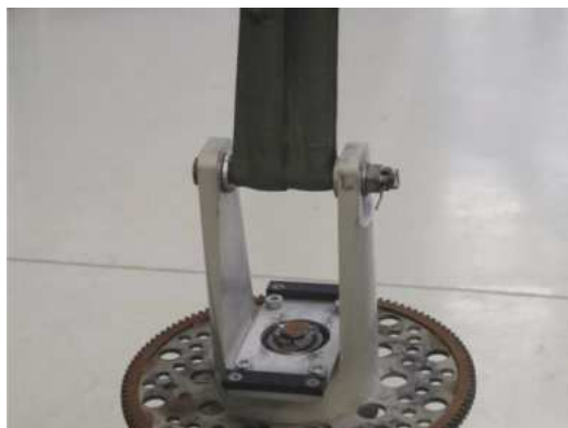
Figure 1 - Lifting belt looped around teeter bolt
