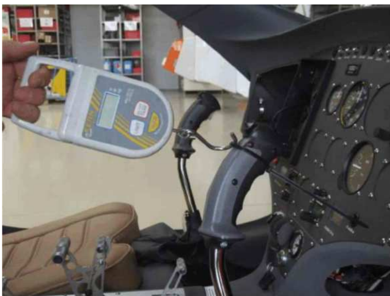
Figure 1 – Measurement of Rotor Control Friction
