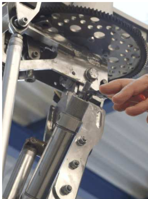
Figure 2 - Remove circlip / snap ring
