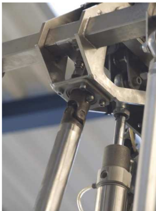
Figure 4 - Re-connect ball joint and upper cardan hinge
