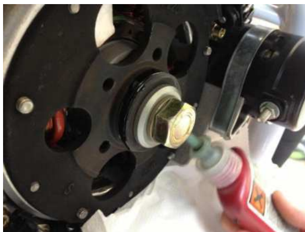
Figure 4 – Loctite 648 on inner and outer thread
