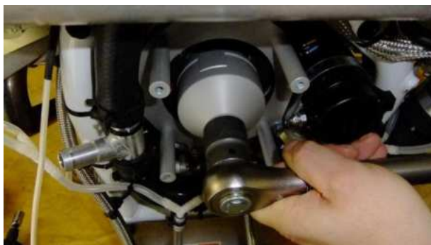
Figure 5 – Torque Dog Gear with 140 Nm
