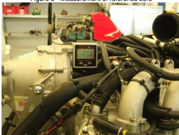
Figure 4 - Measurement of thrust line angle
