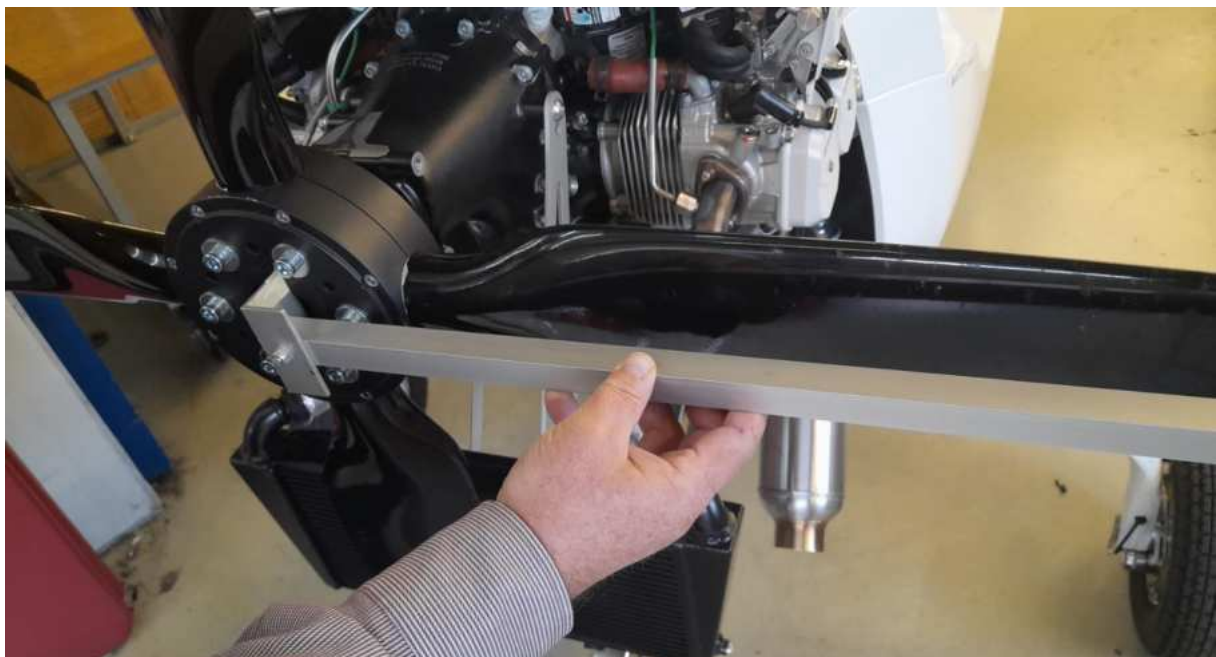
Figure 2 - Propeller pitch adjustment and tool
