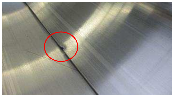
Figure 4 – damage on trailing edge
