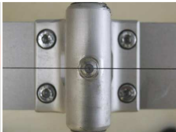
Figure 3 - Reference point at grease nipple
