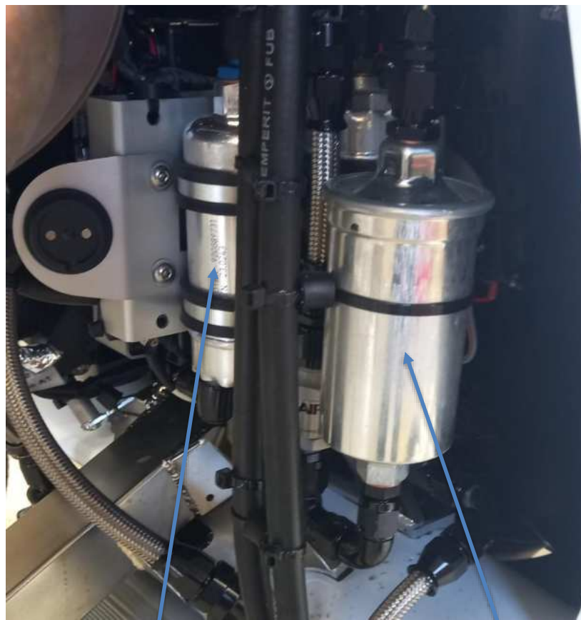
Figure 2 - Location of fuel pumps (within this box) and quick-change fuel filter (916 engine)
