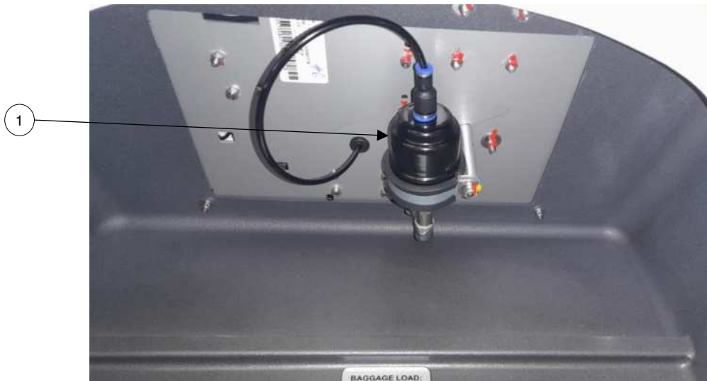
Figure 2 - Location of Filter / Dryer
