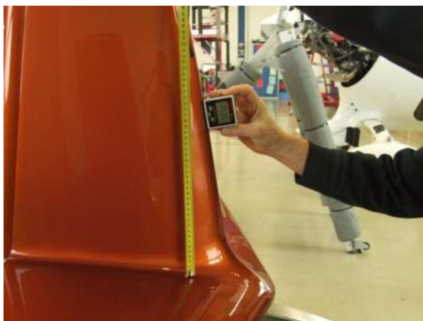
Figure 5 - Measurement of stabilizer incident
