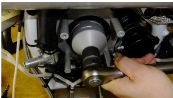
Figure 5 – Torque Dog Gear with 140 Nm
