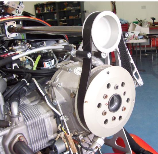
Engine gearbox flange with top hat spacers fitted
