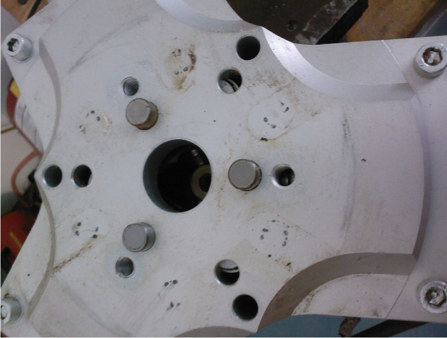
Fit three dowel pins in place (torque transmission between hub and spacer plate)
