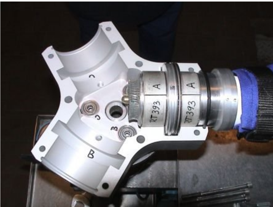
First blade fitted. Ensure the correct blade is mated into the correct hub slot!
