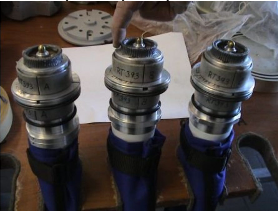
Grease gears before re installation with Aeroshell 5, MIL - G - 3514C.
