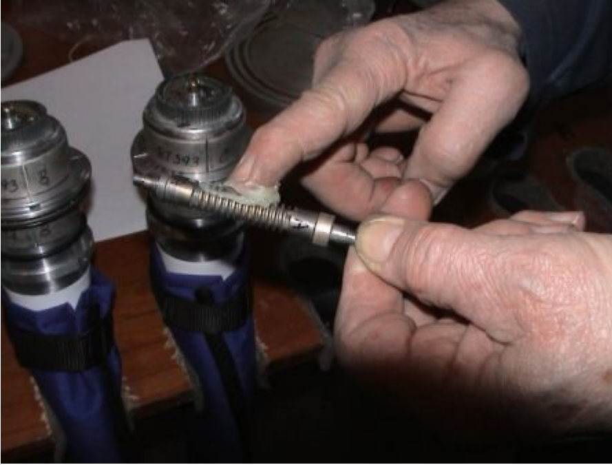
Grease worms before re-installation with Aeroshell 5, MIL - G - 3514C.
