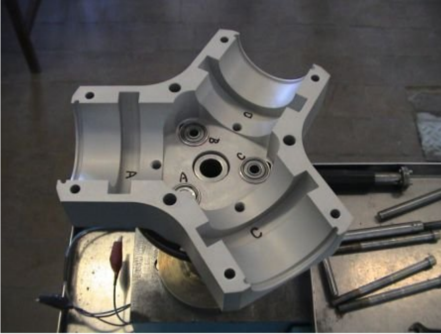
Inside of housing, with worm gear bearings installed
