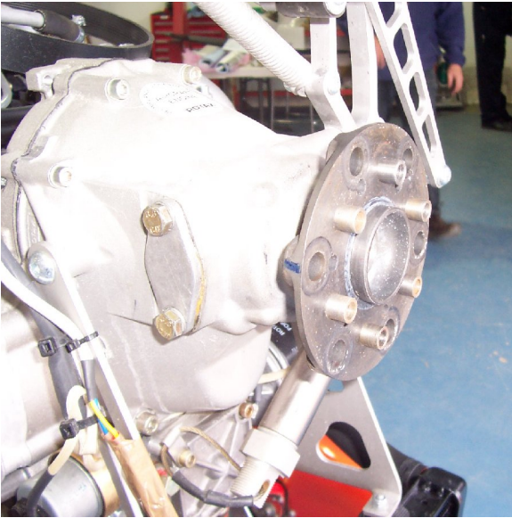
Engine gearbox flange with top hat spacers fitted
