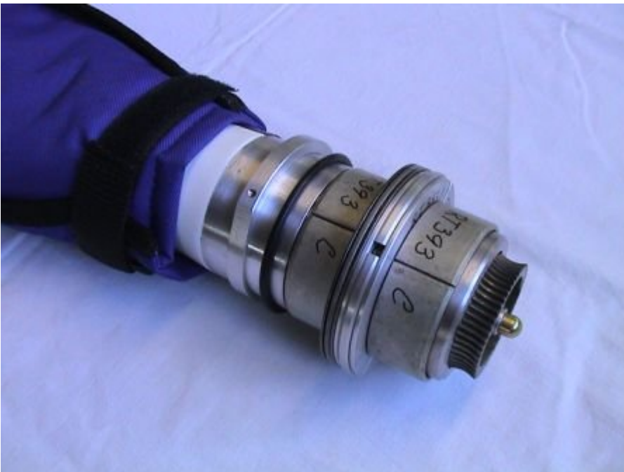
Blade end, fully assembled with bushes and worm gear, and axial pin fitted
