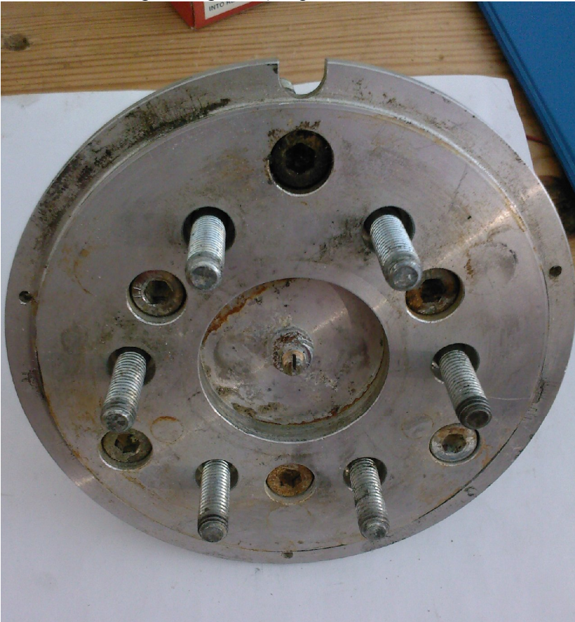
View of flange, engine face, with bolts fitted. Bolts are M8x40 grade 8.8
