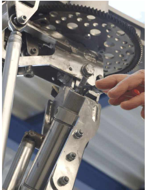
Fig. 4 - Re-connect ball joint and upper cardan hinge
