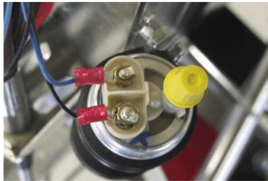
Fig. 5 - El. fuel pump terminal
