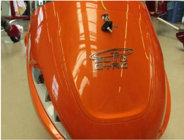
Fig. 1 - Access to dryer / nose compartment closed
