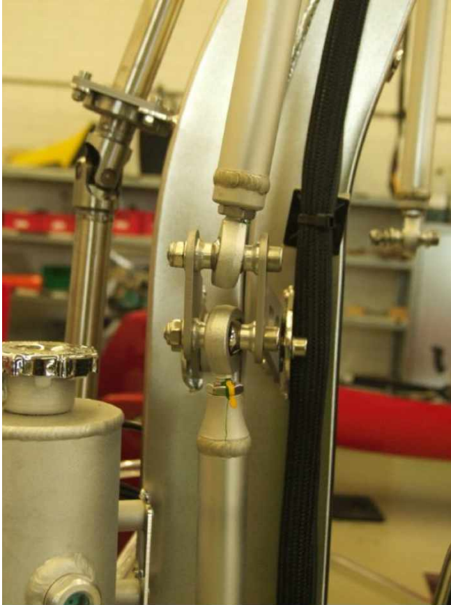
Fig. 2 - Connection of upper ball joint of lower RH flight control rod with bell crank(step3/5)
