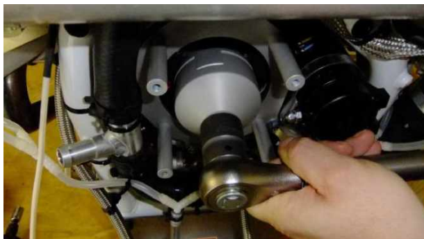
Fig. 5 - Torque dog gear with 140 Nm
