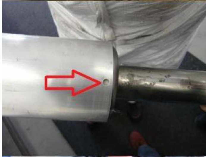
Fig. 5 - Rivets at the cold end of muffler tube
