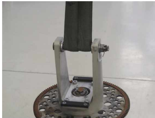
Fig. 1 - Lifting belt looped around teeter bolt
