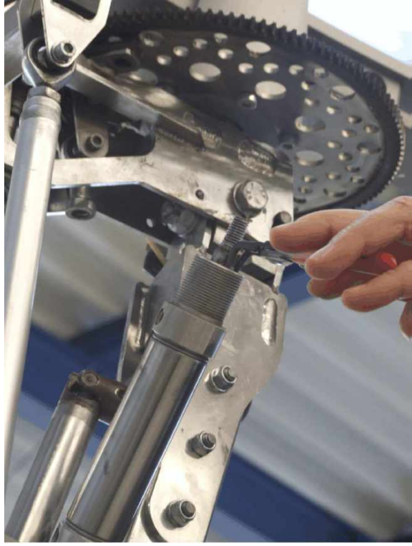
Fig. 2 - Remove circlip / snap ring (step 6)
