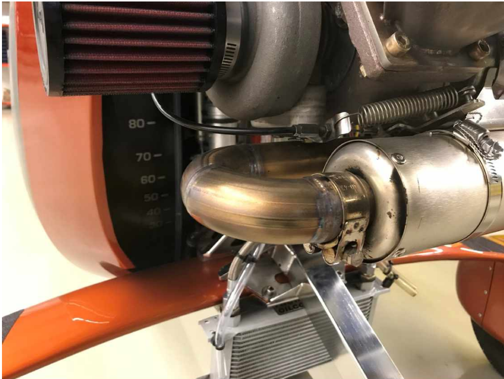
Fig. 1 - Rivets at the hot end and hinge pin clamp (914)
