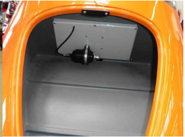
Fig. 1 - Access to dryer / nose compartment opened
