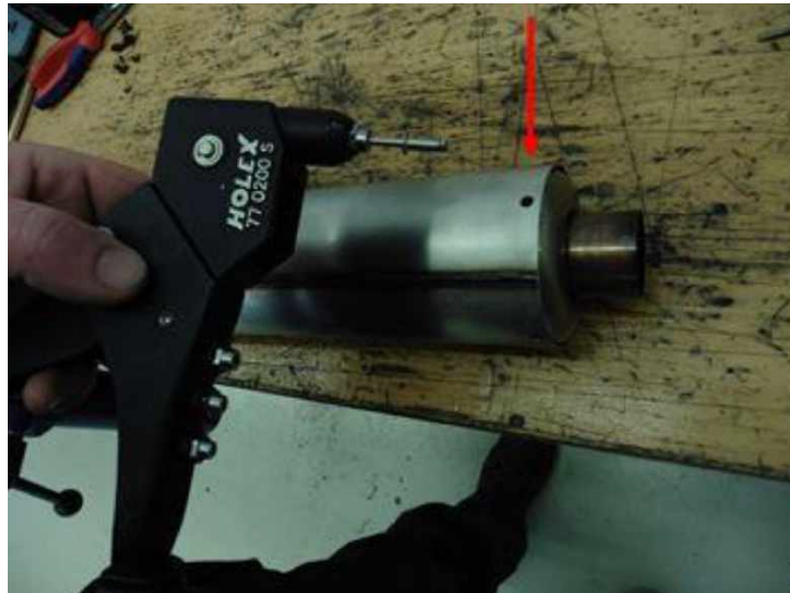
Fig. 6 - Riveting of the outer shell
