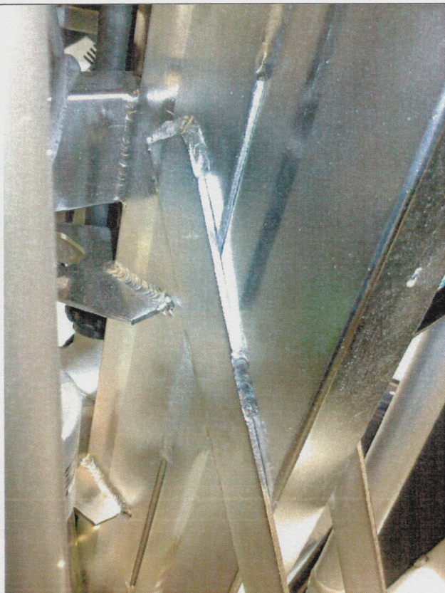
View of welded on strap. Weld as per RSD7178. Use filler metal suitable for stainless steel 1.4301
