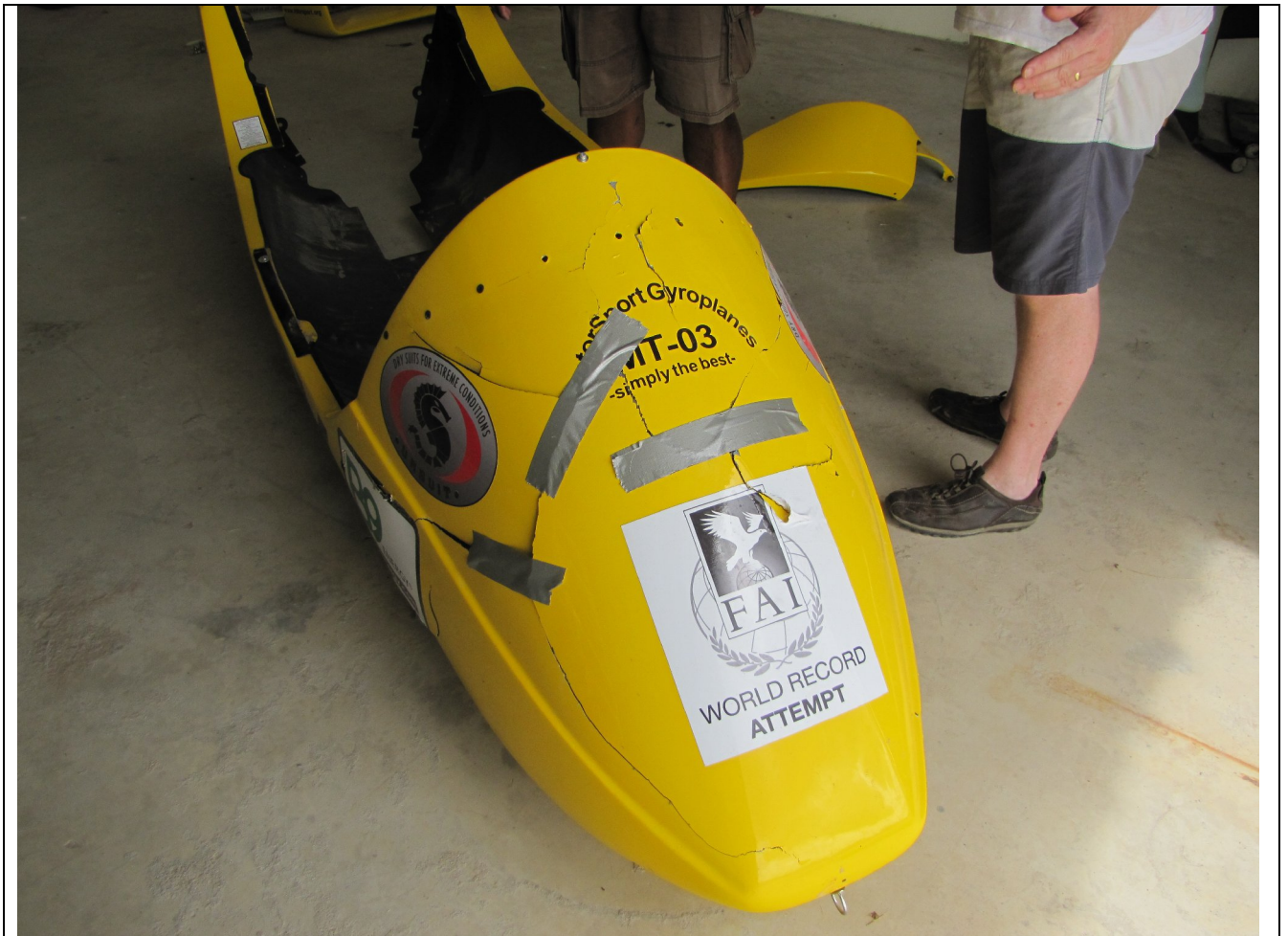
Enclosure nose before repair
