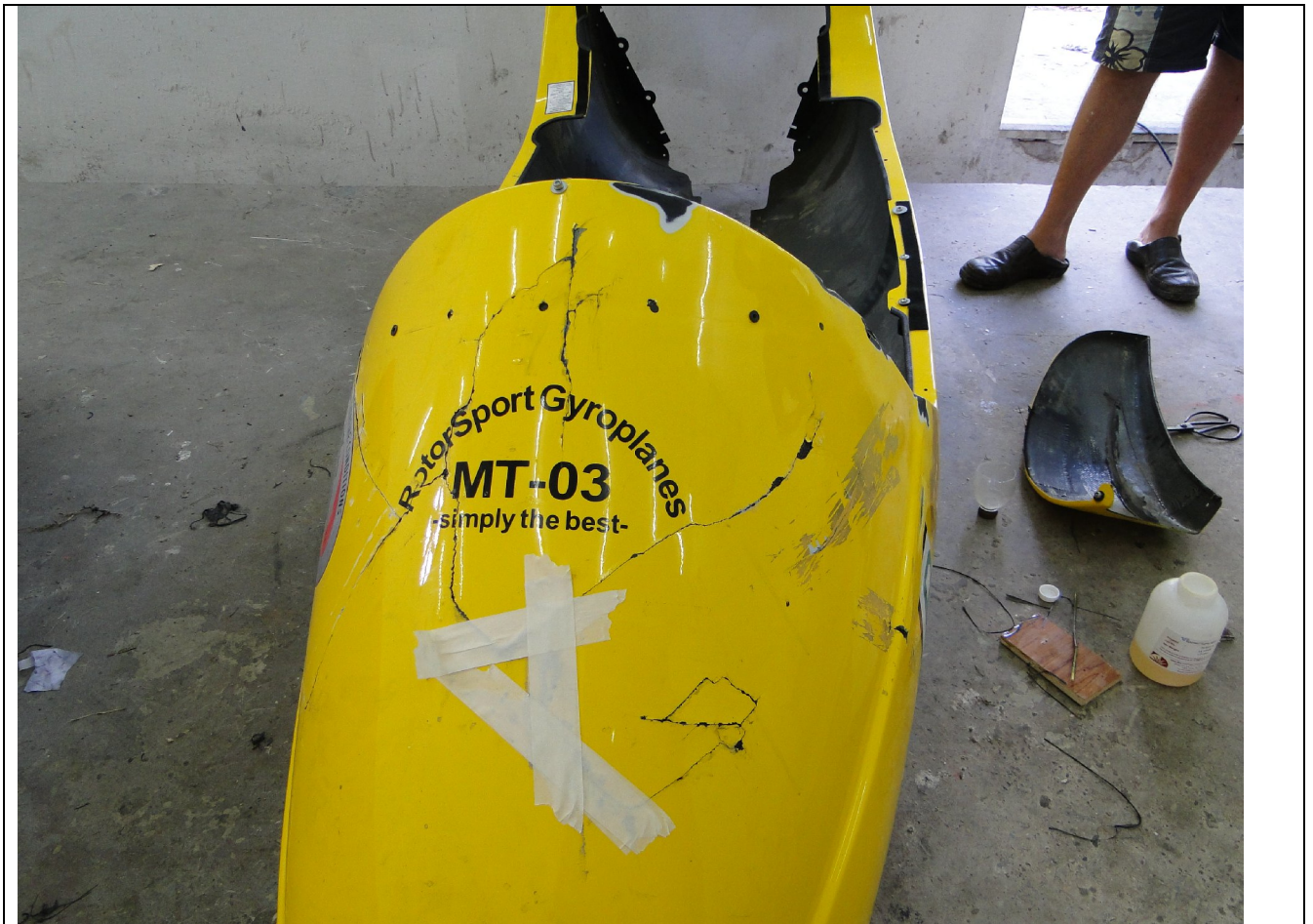
Outside of the nose before repair
