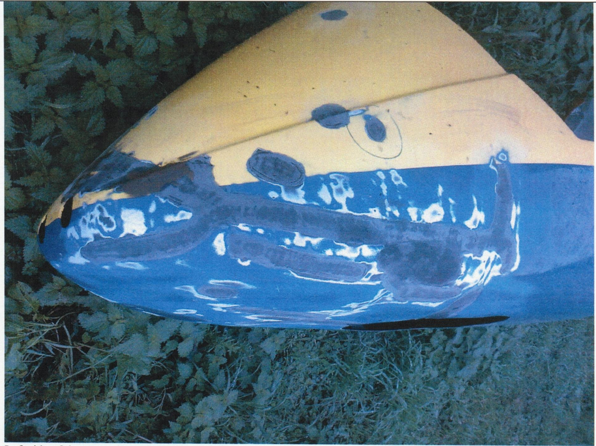
Left side of the nose after repair completion
