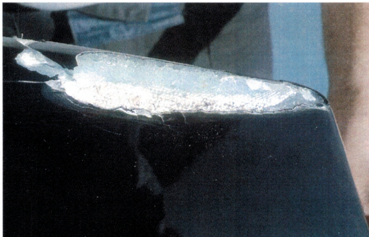
Views of the upper rudder rear edge. This edge is composed mainly of 'Mumba' a type of filler
