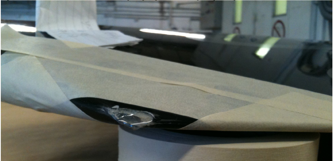
Tip of rudder filled with Wurth ESK -48 for gel repair prior to sanding and painting
