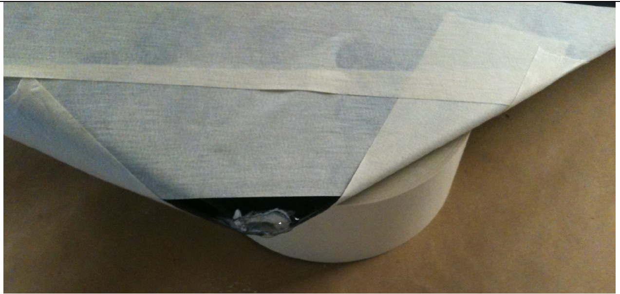
Tip of rudder filled with Wurth ESK -48 for gel repair prior to sanding and painting
