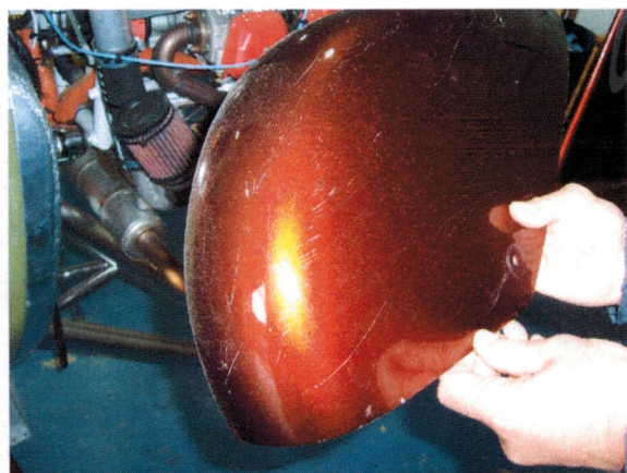
Surface scratches in paintwork
