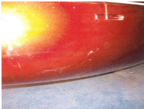
Surface scratches in paintwork
